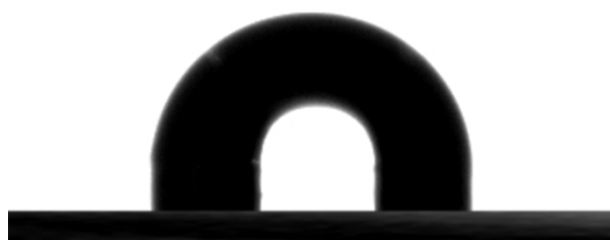
Fig. S5 Water contact angle of poly(BA-mdes)
