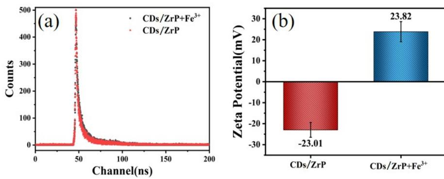
Fig. S8 FL decay spectra (a) and Zeta potential (b) of CDs/ZrP before and after Fe<sup>3+</sup> addition.
