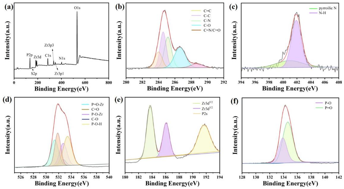
Fig. S1 Full survey (a) and high-resolution XPS of C<sub>1s</sub> (b), N<sub>1s</sub> (c), O<sub>1s</sub> (d), Zr<sub>3d</sub> (e) and P<sub>2p</sub> (f) of CDs/ZrP composites.
