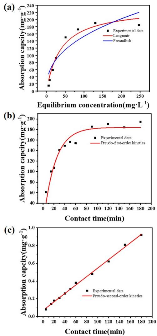
Fig.S6 (a) The adsorption isotherms of ZrP fitted by Langmuir and Freundlich model; (b-c) Adsorption kinetics of ZrP fitted by pseudo-first-order and pseuso-second-order models.
