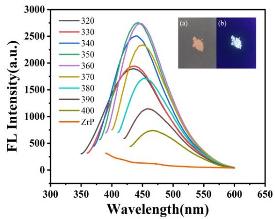
Fig. S4 Fluorescence spectra of CDs/ZrP at  $\lambda_{\text{ex}}=320\sim400$  nm. Inset shows photographs of CDs/ZrP under visible light (a) and 365 nm UV beam (b).
