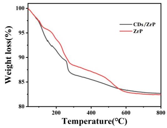
Fig. S3 The TG curves of ZrP and CDs/ZrP composites.
