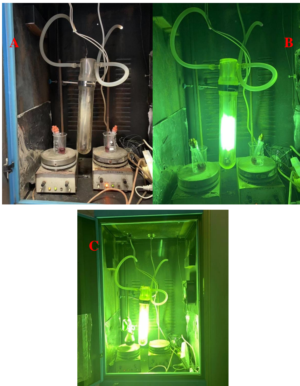
Figure S2. Reaction set-up. Ultraviolet high-pressure Hg lamp as UV-light irradiation (UV \lambda = 365 nm)
