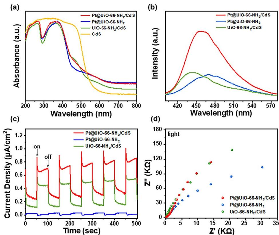
**Fig. S3** (a) UV-vis absorption spectra of Pt@UiO-66-NH<sub>2</sub>/CdS, Pt@UiO-66-NH<sub>2</sub>, UiO-66-NH<sub>2</sub>/CdS and CdS; (b) photoluminescence spectra, (c) transient photocurrent response and (d) EIS Nyquist plots at light of Pt@UiO-66-NH<sub>2</sub>/CdS, Pt@UiO-66-NH<sub>2</sub> and UiO-66-NH<sub>2</sub>/CdS.
