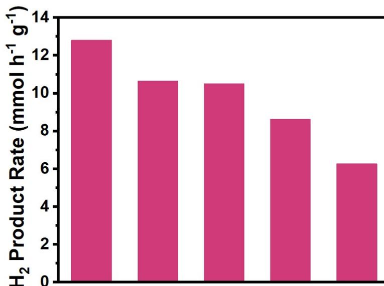
**Fig. S5** five continuous cycles of photocatalytic H<sub>2</sub> production of Pt@H-UiO-66-NH<sub>2</sub>/CdS.
