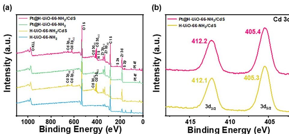
**Fig. S4** (a) XPS survey spectrum H-UiO-66-NH<sub>2</sub>, H-UiO-66-NH<sub>2</sub>/CdS, Pt@H-UiO-66-NH<sub>2</sub> and Pt@H-UiO-66-NH<sub>2</sub>/CdS; high resolution XPS survey spectrum of (b) Cd 3d.
