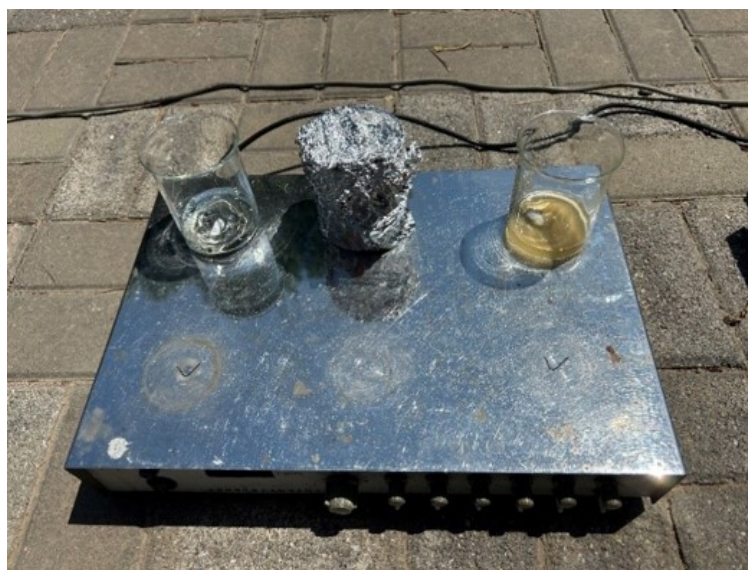
Fig. S8 The experimental diagram of photocatalytic Cr(VI) reduction under real sunlight irradiation.
