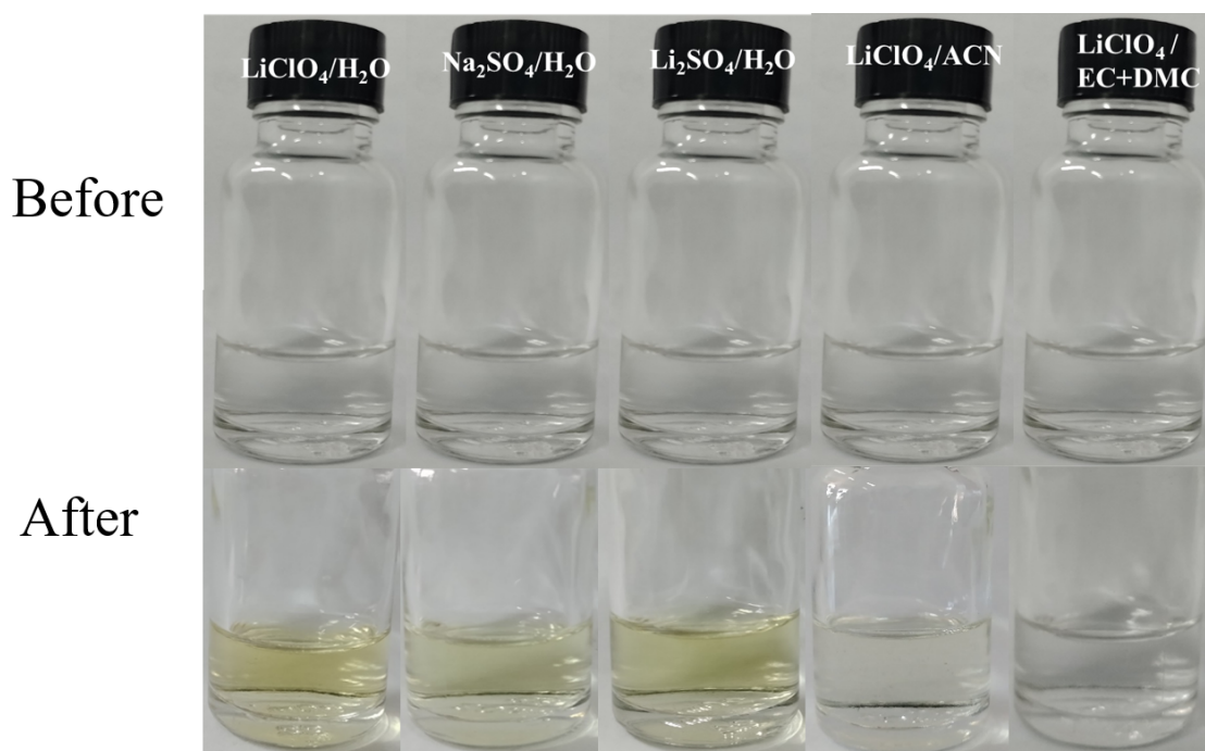
Fig. S3. The digital camera diagram of V_2O_5 before and after electrochemical measure in different electrolytes.
