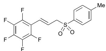
**(E)-1,2,3,4,5-pentafluoro-6-(3-tosylprop-1-en-1-yl)benzene (3i).** Prepared from 1-allyl-2,3,4,5,6-pentafluorobenzene (83 mg, 0.4 mmol) and sodium 4-methylbenzenesulfinate (71 mg, 0.6 mmol, 1.5 equiv) according to general procedure B. White solid (95 mg, 65%), melting point: 149 °C, ratio (single adduct)
