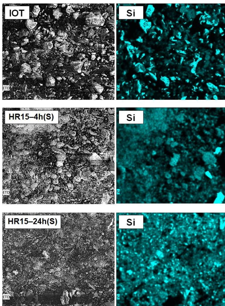
**Figure S3.** EDS mapping for Si of the IOT and of the solid fractions HR15-4h(S) and HR15-24h(S).
