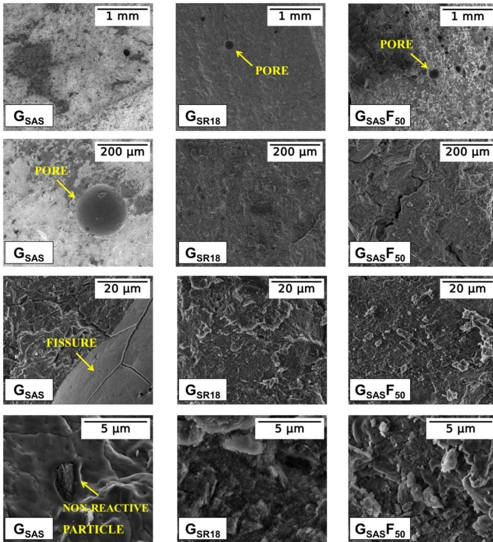
Figure S5. SEM images of  $G_{SAS}$ ,  $G_{SR18}$  and  $G_{SAS}F_{50}$  geopolymers.
