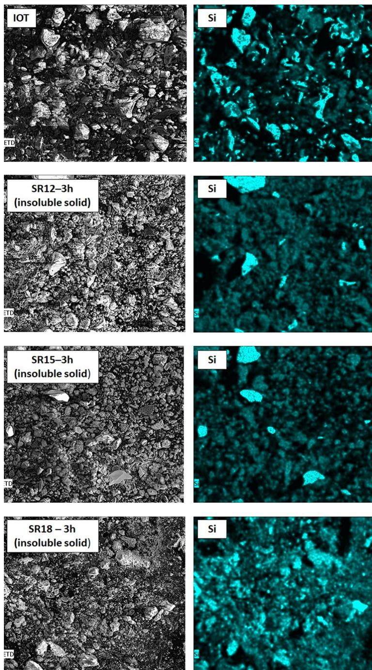
**Figure S4.** EDS mapping for Si of the IOT and residual insoluble solid fractions from SR12-3h, SR15-3h and SR18-3h.
