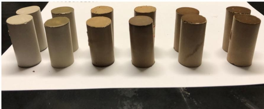
**Figure S1.** Geopolymers produced and demolded after 72 hours.
