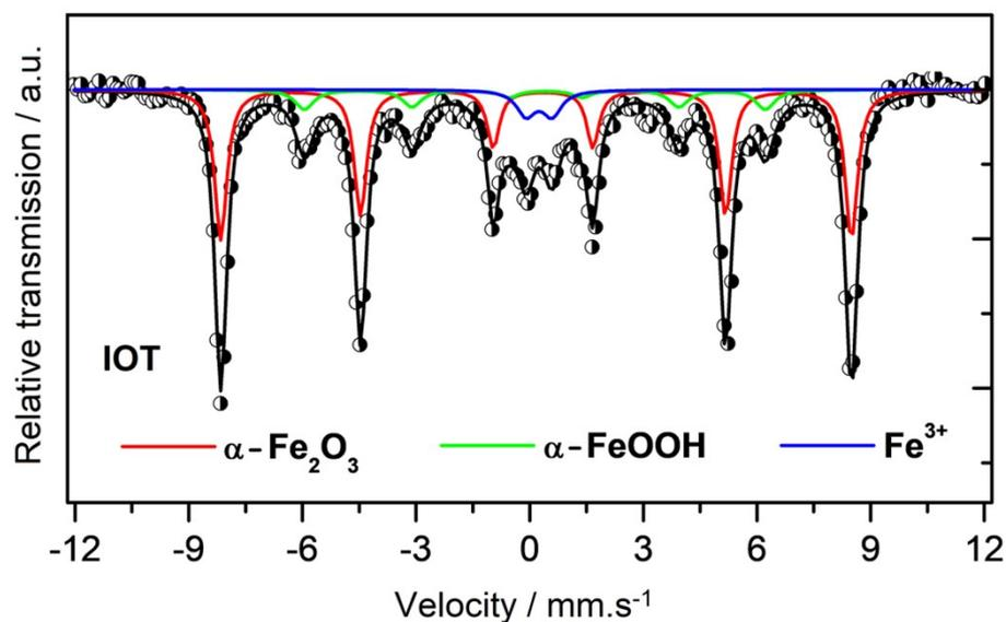
**Figure S2.** Mössbauer spectrum of <sup>57</sup>Fe obtained at room temperature for the IOT.
