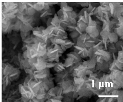
Fig. S8 The SEM image of the CuO@NiCo LDH NSAs electrode after stability test.
