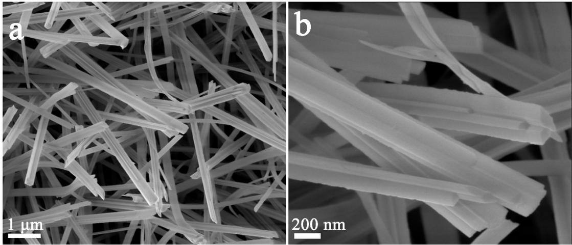
Fig.S1 The SEM image of Cu(OH)<sub>2</sub> NR/CF
