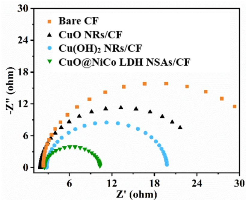
Fig. S5 Nyquist diagram of bare CF, Cu(OH)<sub>2</sub> NRs/CF, CuO NRs/CF and CuO@NiCo LDH NSAs/CF in 0.1 M NaOH dripping with 1 mM glucose.
