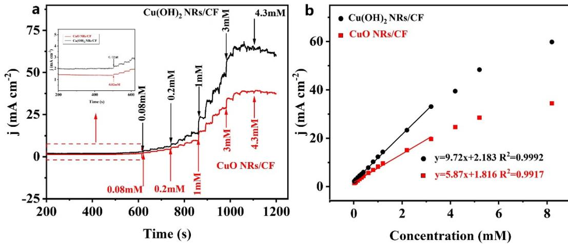
Fig. S6 (a) Amperometric responses of Cu(OH)<sub>2</sub> NRs/CF and CuO NRs/CF with successive additions of glucose to 0.1 M NaOH at 0.7 V. (b) Corresponding linear fitting relationship for Cu(OH)<sub>2</sub> NRs/CF and CuO NRs/CF electrodes.
