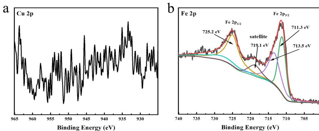
**Figure S6** high-resolution XPS spectra of the recycled catalyst's Cu 2p (b) and Fe 2p (c).
