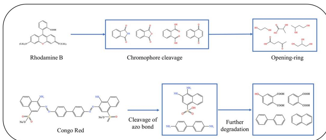
**Figure S7** Probable mechanism for degradation of Rhodamine B and Congo Red.
