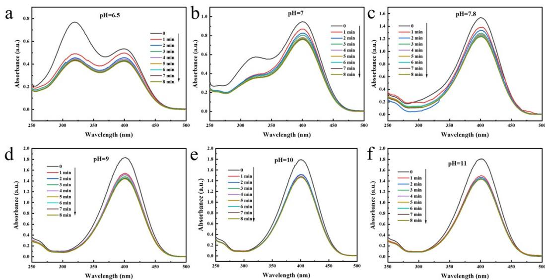
**Figure S5** UV-Vis spectra of 4-NP degradation at different pH in the presence of CFO/AC-2 (1:1).
