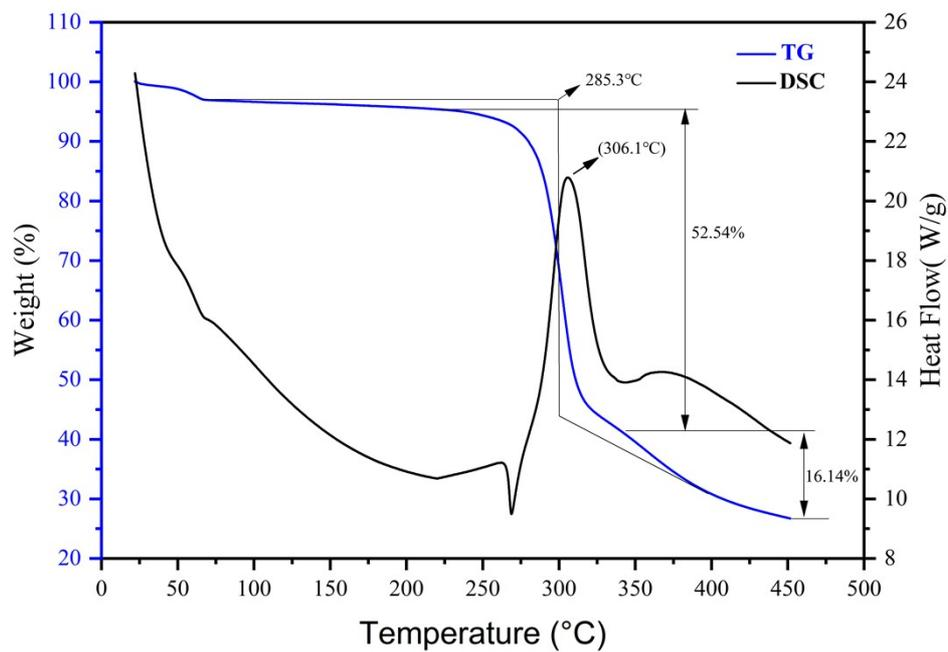
Figure S7 DSC-TG curves of **GD-1** (10 °C/min)
