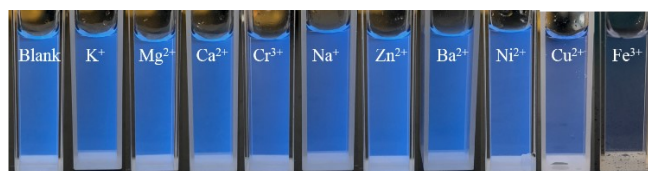
Fig. S7 Fluorescence photos of different metal ions detected by N-CQDs
