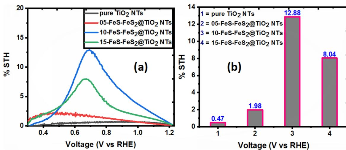
Figure S6. (a) %STH curves (b) %STH Histogram of pure TiO<sub>2</sub> NTs, 05-FeS-FeS<sub>2</sub>@TiO<sub>2</sub> NTs, 10-FeS-FeS<sub>2</sub>@TiO<sub>2</sub> NTs and 15-FeS-FeS<sub>2</sub>@TiO<sub>2</sub>@TiO<sub>2</sub> NTs
