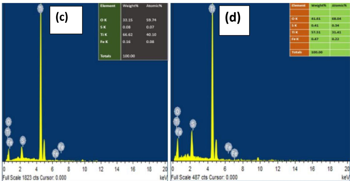
**Figure S2. EDS spectrum of (a) 10-FeS-FeS<sub>2</sub>@TiO<sub>2</sub> NTs (b) 15-FeS-FeS<sub>2</sub>@TiO<sub>2</sub> NTs, (c) 10-FeS-FeS<sub>2</sub>@TiO<sub>2</sub> NTs and (d) 15-FeS-FeS<sub>2</sub>@TiO<sub>2</sub> NTs**
