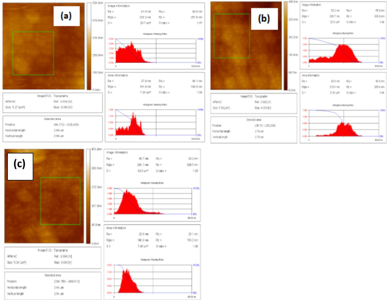
Figure S3 AFM images showing surface roughness of (a) pure  $\text{TiO}_2$  NTs (b) 10-FeS- $\text{FeS}_2$ @ $\text{TiO}_2$  NTs (c) 15-FeS- $\text{FeS}_2$ @ $\text{TiO}_2$  NTs
