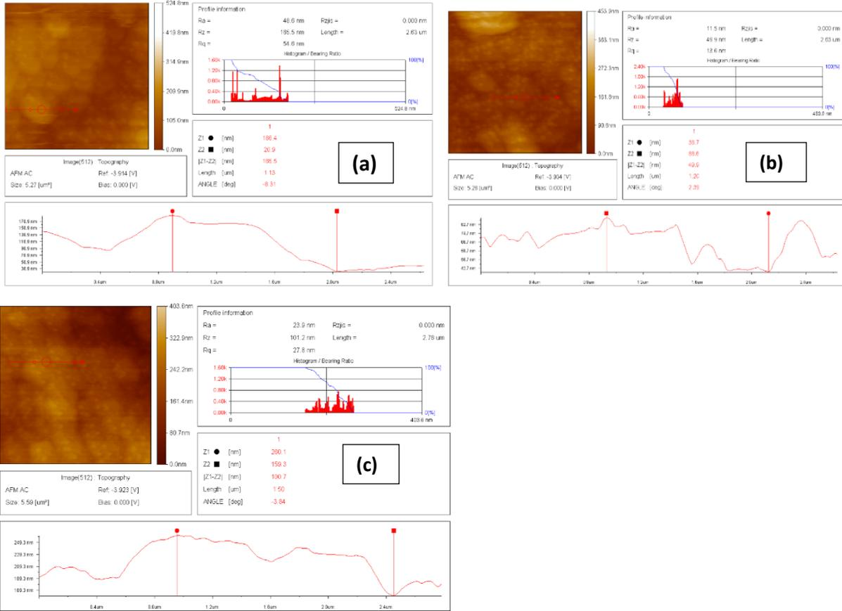
**Figure S4 AFM images showing surface thickness of (a) pure TiO<sub>2</sub> NTs, (b) 10-FeS-FeS<sub>2</sub>@TiO<sub>2</sub> NTs and (c) 15-FeS-FeS<sub>2</sub>@TiO<sub>2</sub> NTs**
