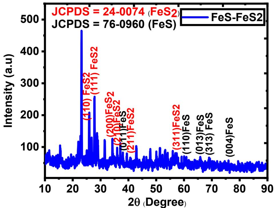
Figure S1. XRD of 50 SILAR cycles of FeS-FeS<sub>2</sub>
