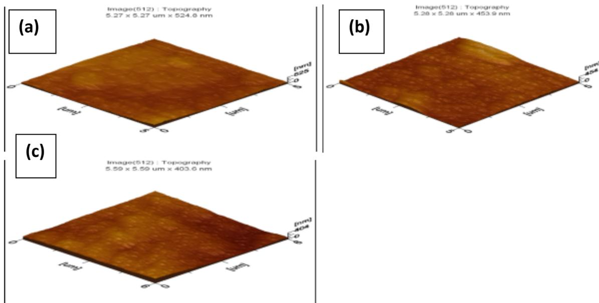
Figure S5 AFM images showing topography of (a) pure TiO<sub>2</sub> NTs (b) 10-FeS-FeS<sub>2</sub>@TiO<sub>2</sub> NTs (c) 15-FeS-FeS<sub>2</sub>@TiO<sub>2</sub> NTs
