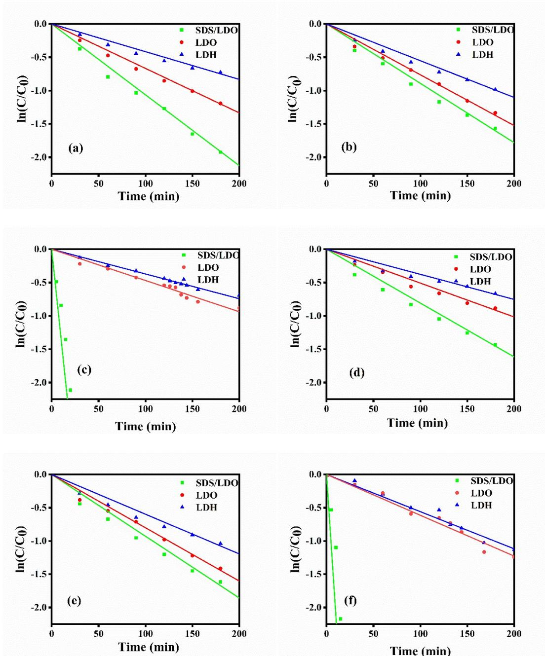
**Fig. S4.** Pseudo-first-order kinetic equation for catalytic degradation of Nap and PA
