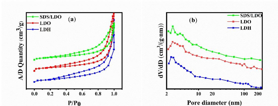
**Fig. S2.**  $N_2$  adsorption/desorption isotherm of catalysts (a) and Pore size distribution curves (b).
