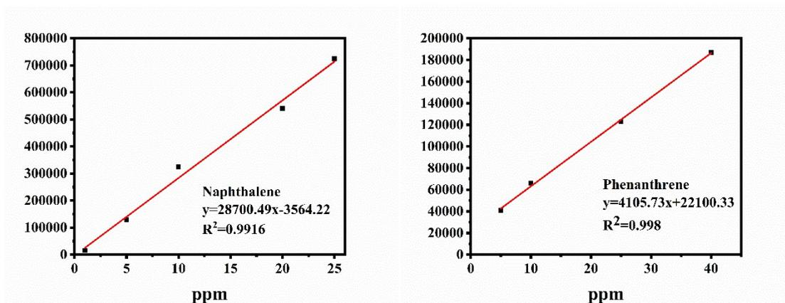
Fig. S1. Standard curve of Nap and PA.
