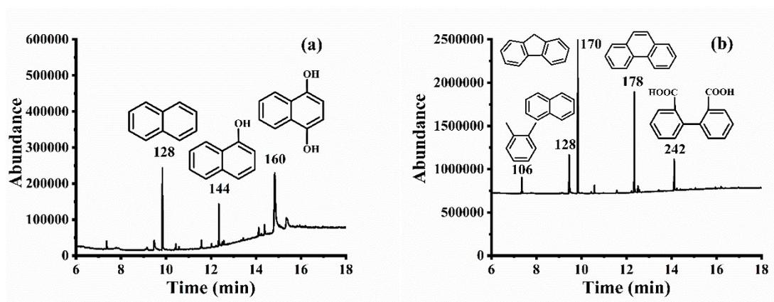
Sch. S1. Degradation mass spectrometry (a) Nap and (b) PA.
