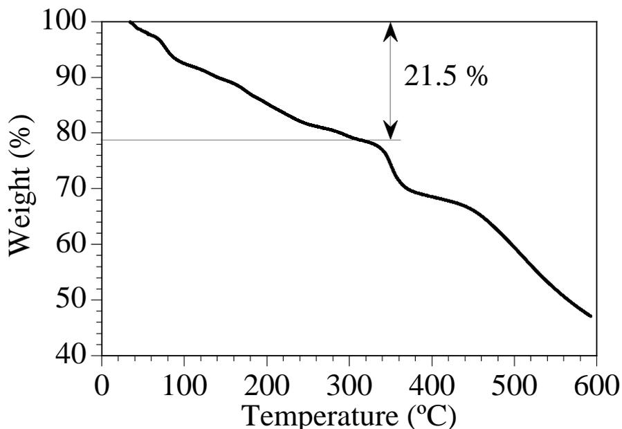
**Figure S4.** Thermogravimetric analysis of compound **1** in the temperature range 20-600 °C.
