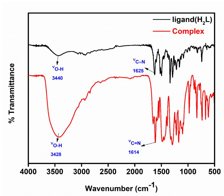
**Figure S1.** FT-IR spectra of the H<sub>2</sub>L ligand and of compound **1**.
