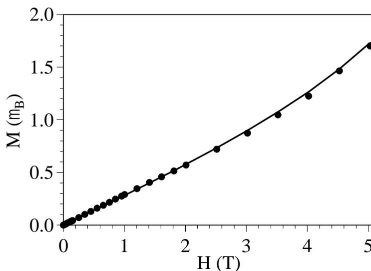
**Figure S7.** Isothermal magnetization of compound **1** at 2 K. Solid line is the best fit to the model
