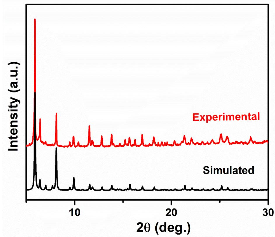
Figure S3. Experimental and simulated powder XRD pattern for compound 1.
