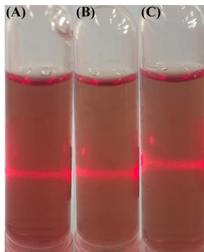
Figure S3. Digital photos of (A) SA 12.0 C 0.5 PS, (B) SA 12.0 C 0.7 PS and (C) SA 12.0 C 0.9 PS solutions with laser irradiation.
