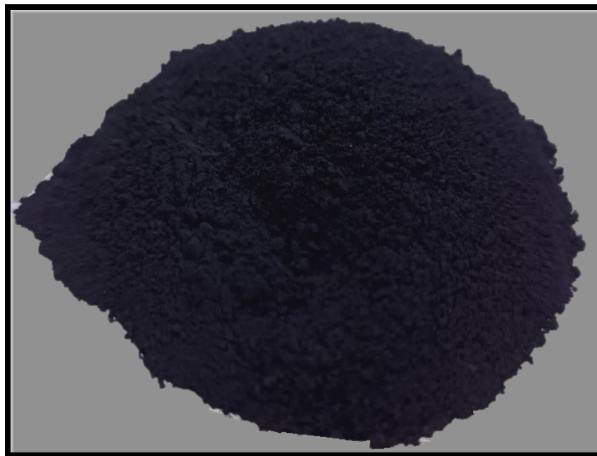
Fig.S2. Digital image of AC/Ppy/CuPC nanocomposite
