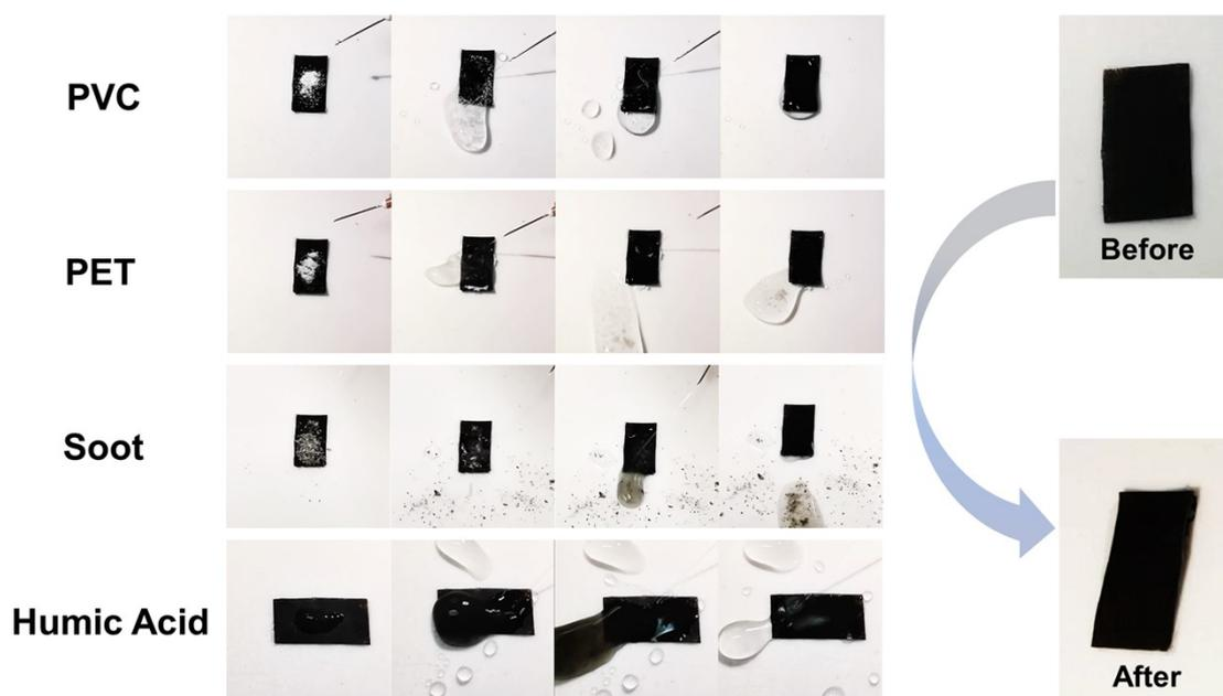
Figure S8. The pollution resistance performance of PTFE-R-O to different simulated solid waste.
