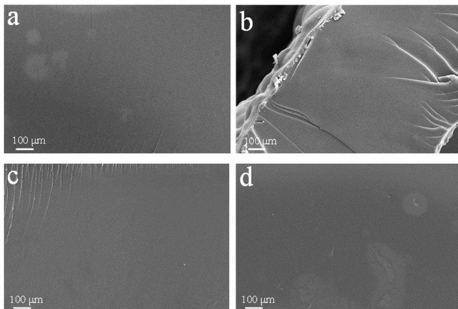
Fig.S3. Cross-section SEM images of the hydrogel membranes obtained after drying, (w polyetherimide: polyvinyl imide = 2:1 (a), 1.5:1 (b), 1:1 (c) and 1:1.5 (d).
