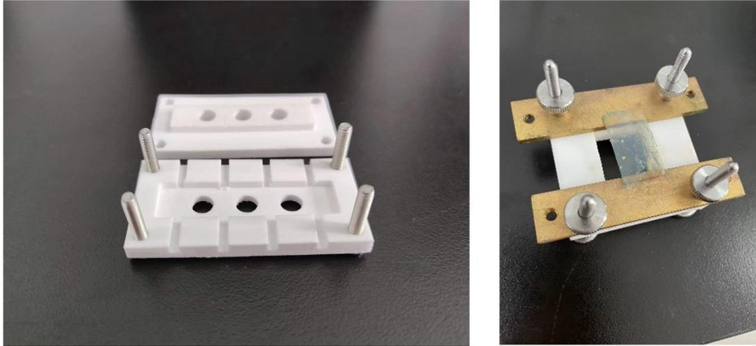
Fig. S5. The photos of four-electrode testing fixture.
