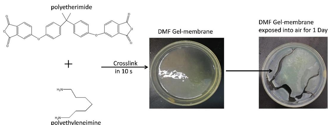
Fig. S1. Schematic diagram of the fabrication process of the novel polyetherimide DMF Gel-membranes.
