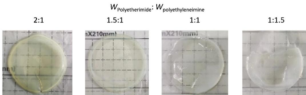
Fig.S2. The photos of the hydrogel membranes with the quality ratio ( $W_{\text{Polyetherimide}} : W_{\text{polyethyleneimine}}$ ) which was set to 2:1, 1.5:1, 1:1 and 1:1.5.
