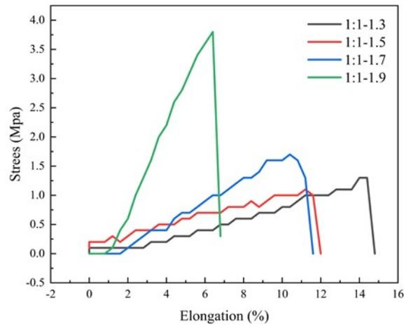
Fig.S6. The tensile testing of the 1:1 hydrogel membrane (The thicknesses are 1.3, 1.5, 1.7, and 1.9mm, respectively).
