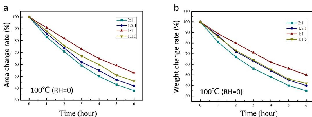
Fig.S4. The water retention capacity of the obtained hydrogel membranes, the change of area (a) and weight (b).
