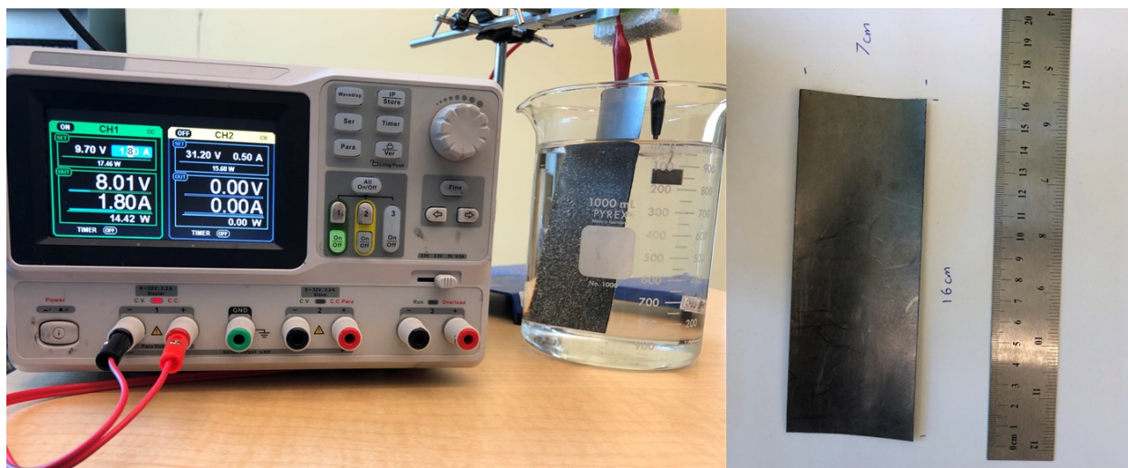
Figure S1: Mass production of GO in 1M nitric acid: 4.2 g of graphite results in 4 g of GO sheets in just 15 min.
