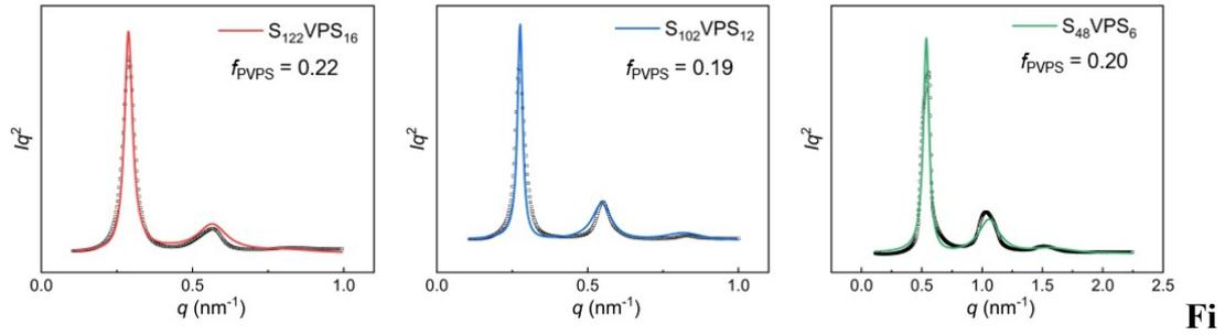
**g. S6** Fitting results of the SAXS profiles. Open squares represent the experimental data and solid lines are the fitting results.
