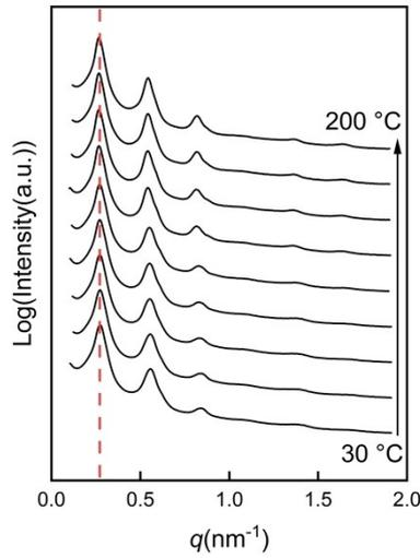
**Fig. S7** Temperature-variable SAXS profiles of  $S_{102}VPS_{12}$ .
