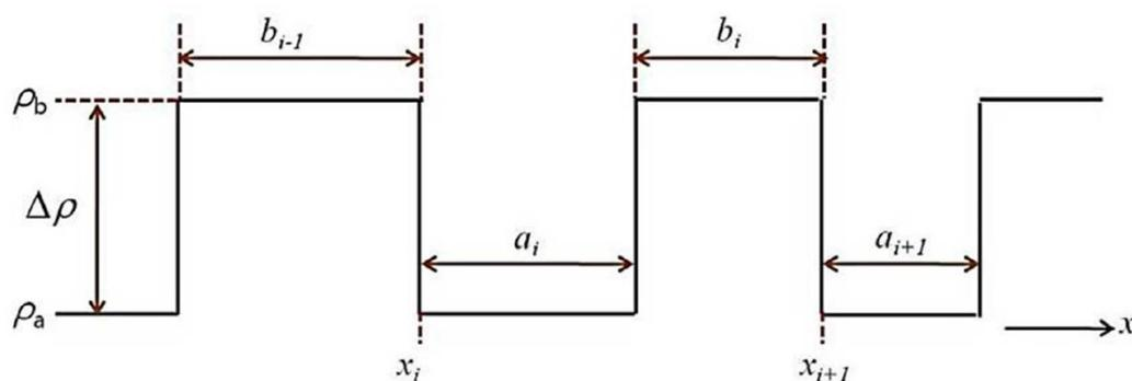
**Fig. S5** Scattering length density profiles in the direction perpendicular to the lamellar plane for the variable lamellar thickness structure model.
