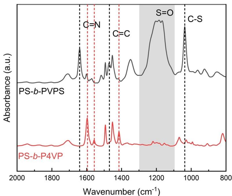
**Fig. S4** FTIR spectra of PS-*b*-P4VP and PS-*b*-PVPS
