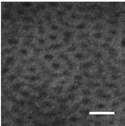
**Fig. S9** TEM image of  $S_{122}VPS_{11}$ . The scale bar is 30 nm.
