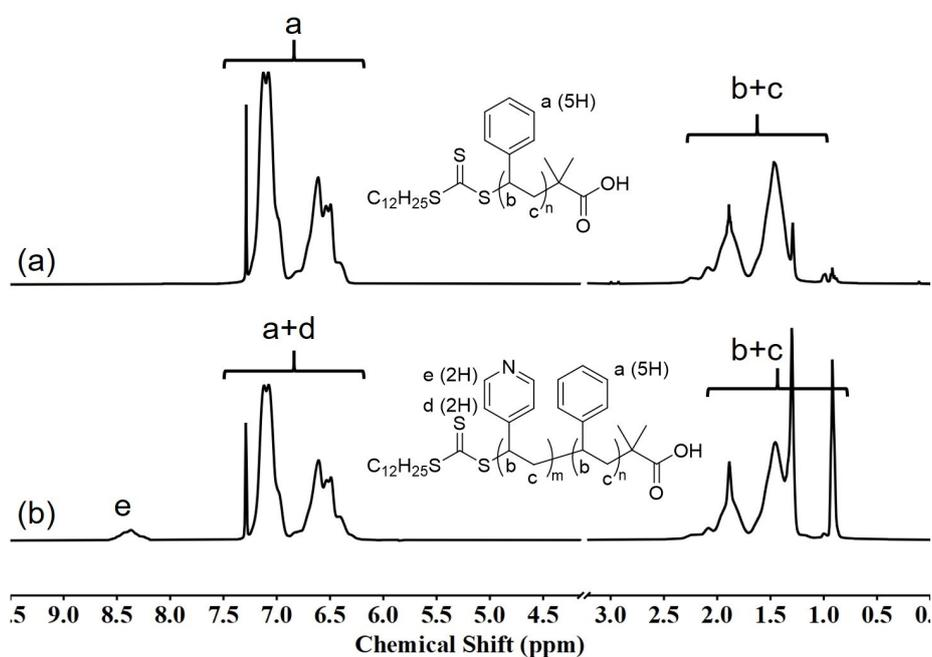
**Fig. S2** Representative <sup>1</sup>H NMR spectra of PS<sub>122</sub>-CTA (a) and S<sub>122</sub>4VP<sub>16</sub> (b) in CDCl<sub>3</sub>.
