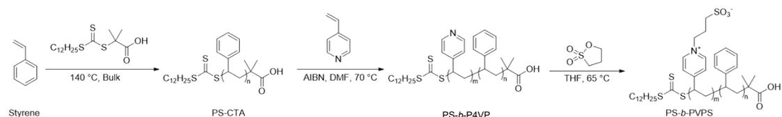
**Fig. S1** Synthetic routine of PS-*b*-PVPS BCPs.
