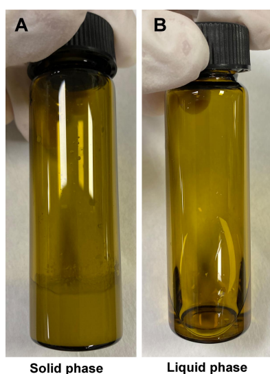
Fig. S1 (A) Solid phase (35 °C) and (B) liquid phase (45 °C) of PCM.
