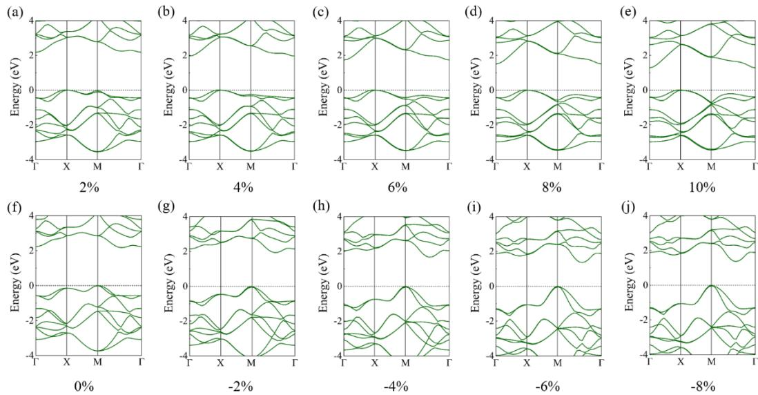
**Fig. S7 (a-j)** Band structure of SnAs<sub>2</sub> under different biaxial strains.
