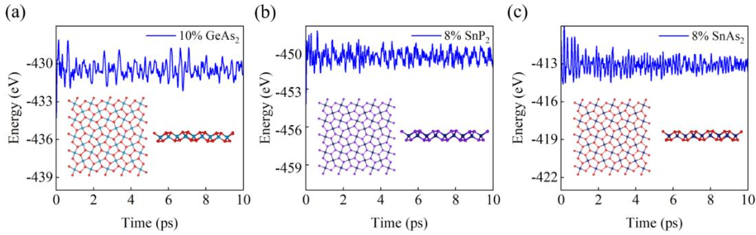
**Fig. S4** Energy fluctuations for strained monolayers GeAs<sub>2</sub> (a), SnP<sub>2</sub> (b), and SnAs<sub>2</sub> (c) by MD simulations at 300 K. The insets are the snapshots taken from the end of each simulation.
