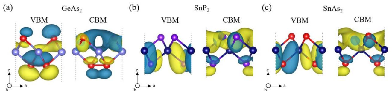
**Fig. S3** The spatial charge density of VBM and CBM of the pentagonal GeAs<sub>2</sub> (a), SnP<sub>2</sub> (b), and SnAs<sub>2</sub> (c). The isolevels are set to be 0.004 eÅ<sup>-3</sup>.
