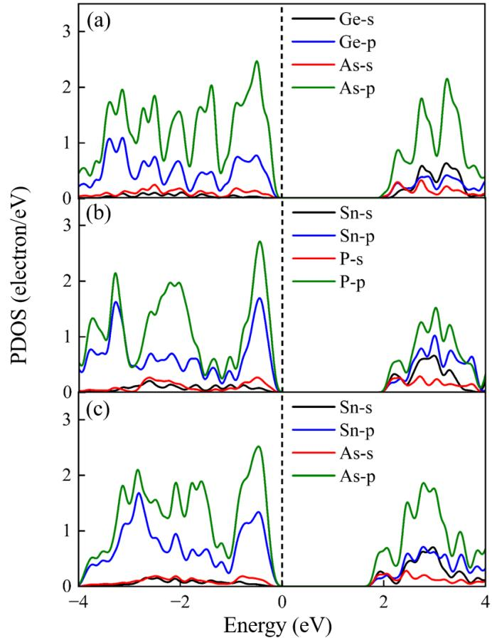
**Fig. S2** The partial density of states (PDOS) of GeAs<sub>2</sub> (a), SnP<sub>2</sub> (b), and SnAs<sub>2</sub> (c).
