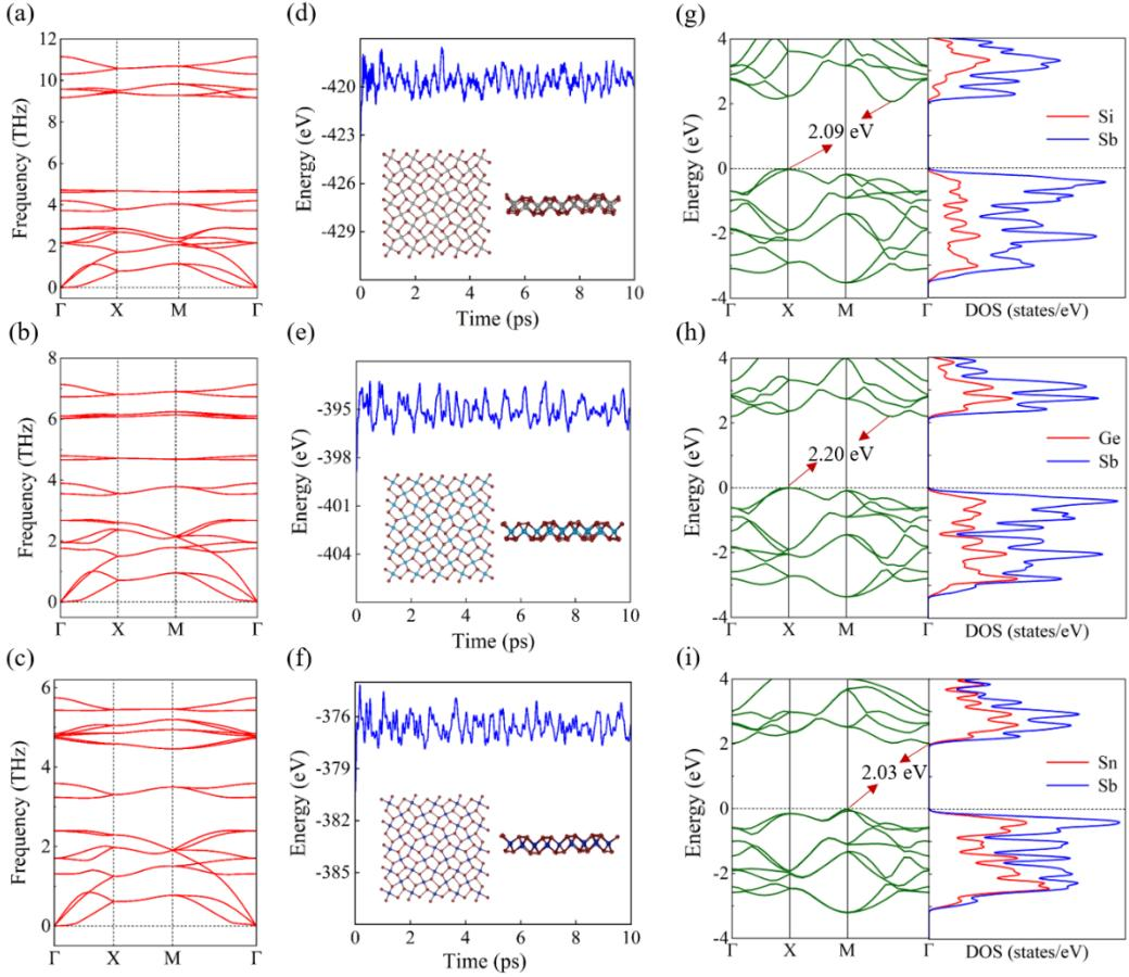
**Fig. S1** The phonon spectra (a-c), Energy fluctuations in AIMD simulations at 300 K (d-f), HSE06 band structures and the corresponding partial density of states (g-i) of SiSb<sub>2</sub>, GeSb<sub>2</sub> and SnSb<sub>2</sub> monolayers. The insets in (d-f) are the snapshots taken from the end of each simulation.
