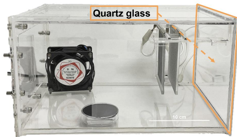
Fig. S9 Photograph of simulated reaction chamber for formaldehyde reaction (quartz glass on the right, 9 L), scale bar, 10 cm.
