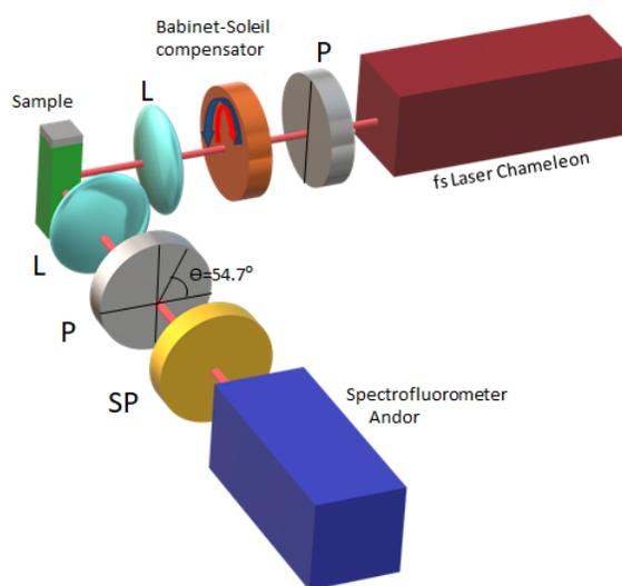
**Figure S6.** A scheme of the FDCD optical set-up (P=polarizer, L=lens, SP=shortpass filter).
