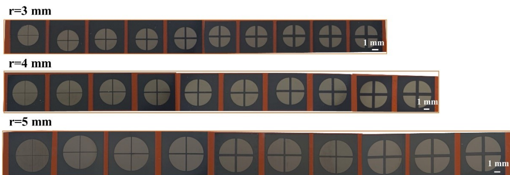
Fig. S10. Composite pattern with different parameters. To test the influencing factors of droplet self-splits, we prepared different SHL radius patterns, in which the stripe spacing of each pattern is from 0.1mm to 1.0 mm.
