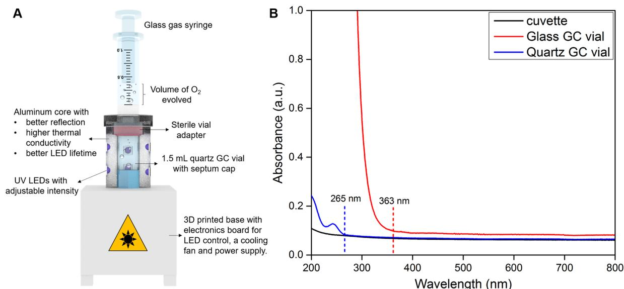
Figure S3: (A) Schematic representation of the setup used for determining the amount of  $\text{O}_2$  evolved (B) UV-vis spectra comparing the absorbance properties of a quartz cuvette, glass GC vial and quartz GC vial.
