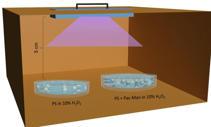
Figure S8: Microplastic degradation setup
