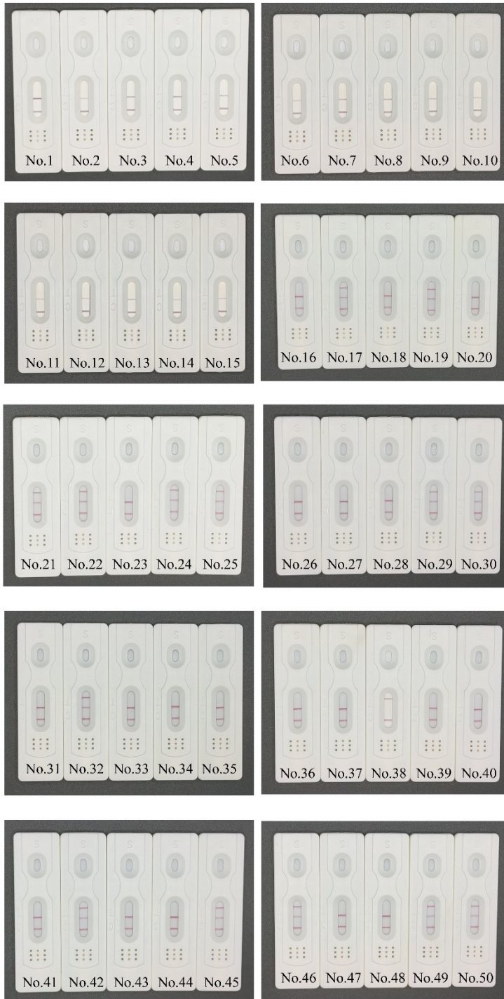
Fig S6. LFTS results of rs671 blood gDNA in 50 cases. (The first 15 results were left for too long, more than four months, and the strips had varying degrees of discoloration.)
