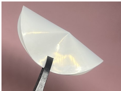
Figure S5. Photo of superhydrophobic filter paper placed for 300 days. per placed for 300 days.
