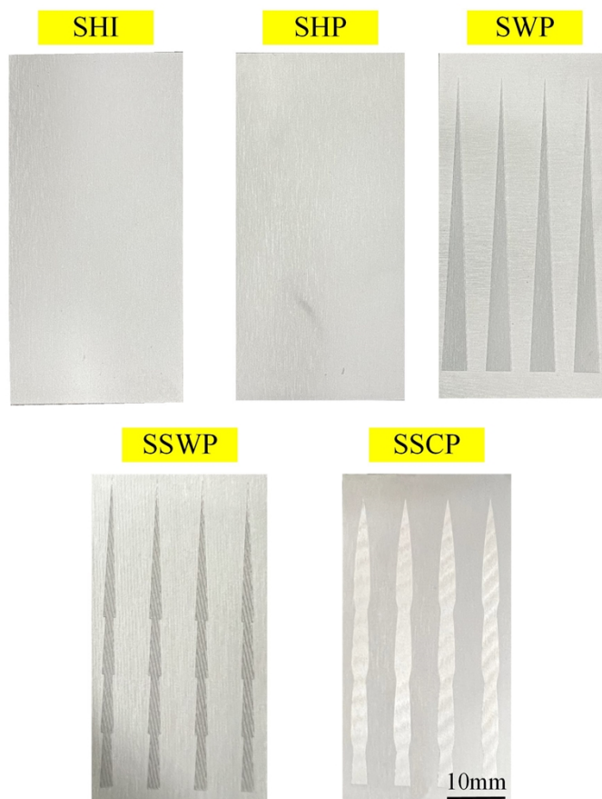
Figure S12. The optical images of the entire superhydrophilic surface (SHI), entire superhydrophobic surface (SHP), superhydrophilic single wedge-shaped pattern (SWP), superhydrophilic serial wedge-shaped pattern (SSWP), and superhydrophilic serial cycloid-shaped pattern (SSCP).
