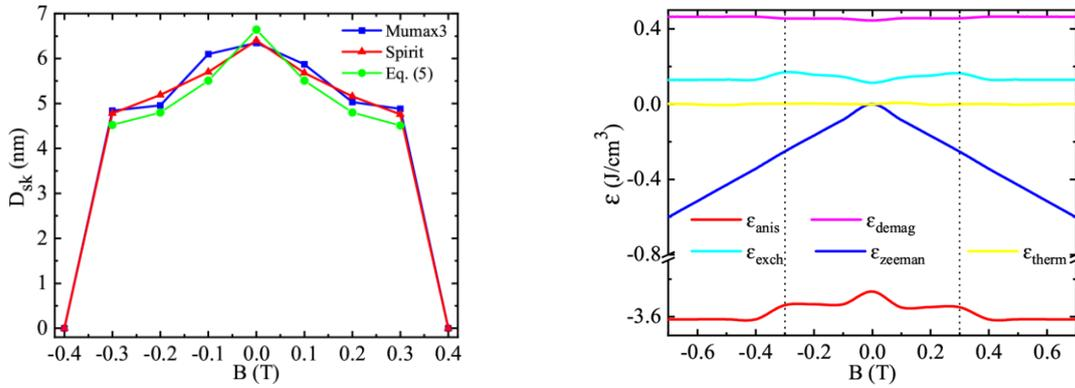
Fig. S4. (left) The evolution of the diameter of skyrmions, obtained by Mumax3 and Spirit respectively, and (right) The magnetic energy density  $\epsilon$  as a function of the external magnetic field  $B$  for MnSeTe.
