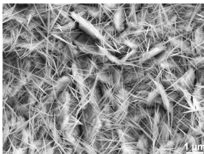
Figure S7 FESEM image of NF@NiCoO 2 NSA@Co 3 O 4 NWA after the stability test.
