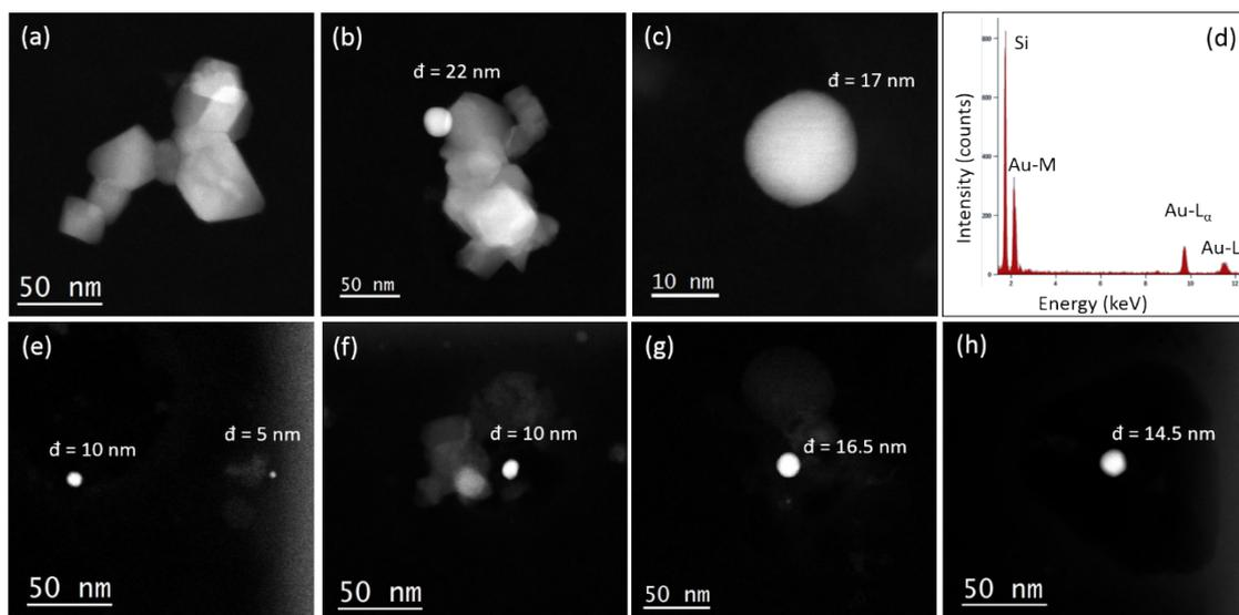
**Figure S2** HAADF –STEM images of AuCZ after O700. (a) Representative image of CZ support aggregate in the absence of Au nanoparticles; (b) agglomerated Au particle attached to CZ support, (c) isolated Au nanoparticle found in the grid membrane and (d) the corresponding XED spectrum. (e - h) examples of single Au particles observed into the grid membrane after O700.
