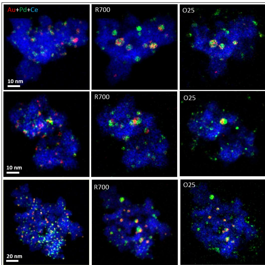
**Figure S5.** Comparison of representative Identical Location HAADF-STEM -XEDS composition maps of AuPdCZ catalysts at three different stages: initial, after R700 and after 30-month of storage under air at room temperature. The maps are represented by signals extracted from Au-L (red), Pd-L (green), and Ce-L (blue).
