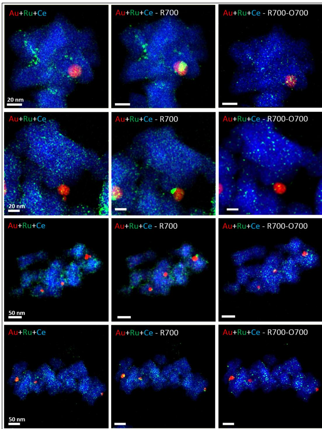
**Figure S6.** Comparison of representative Identical Location HAADF-STEM -XEDS composition maps of AuRuZ catalysts at three different stages: before, after R700 and after O700. The maps are represented by signals extracted from Au-L (red), Ru-L (green), and Ce-L (blue).
