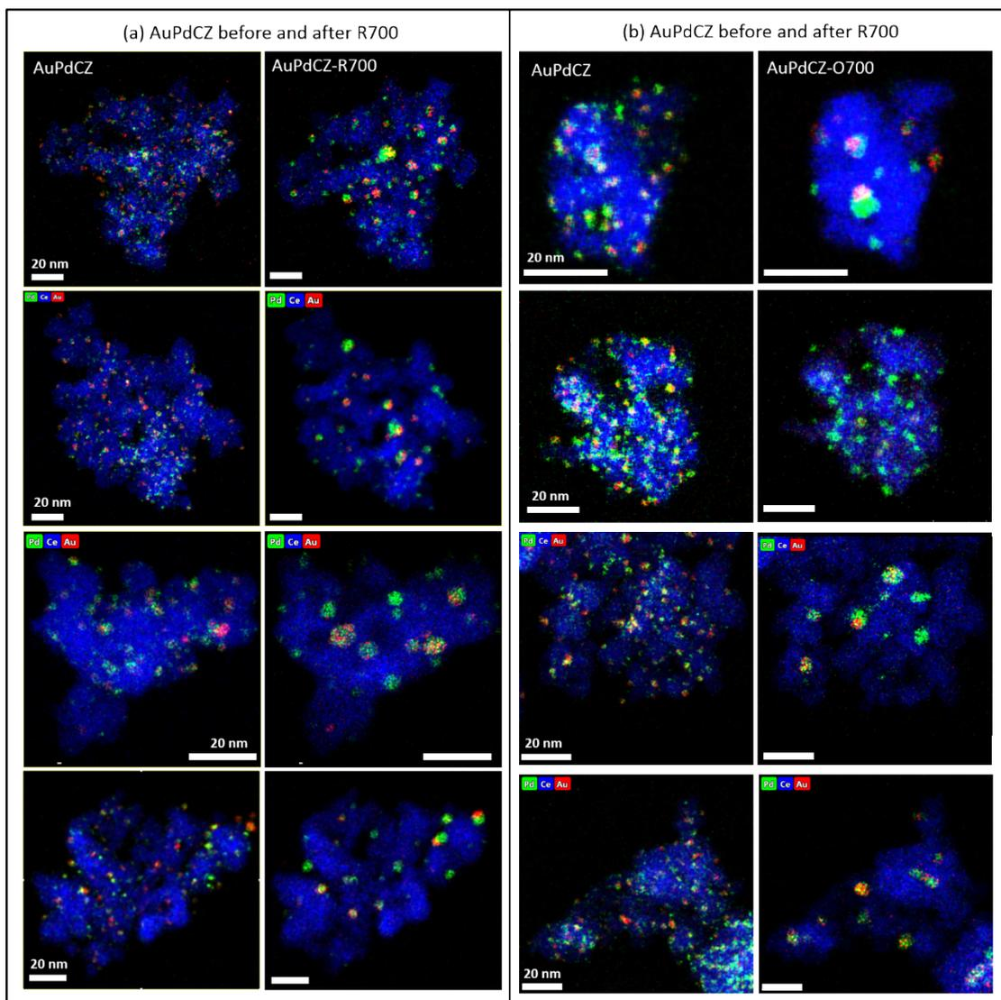
**Figure S3** Representative Identical Location HAADF-STEM -XEDS composition maps of AuPdCZ catalysts (a) before and after R700; (b) before and after O700. The maps are represented by signals extracted from Au-L (red), Pd-L (green), and Ce-L (blue).
