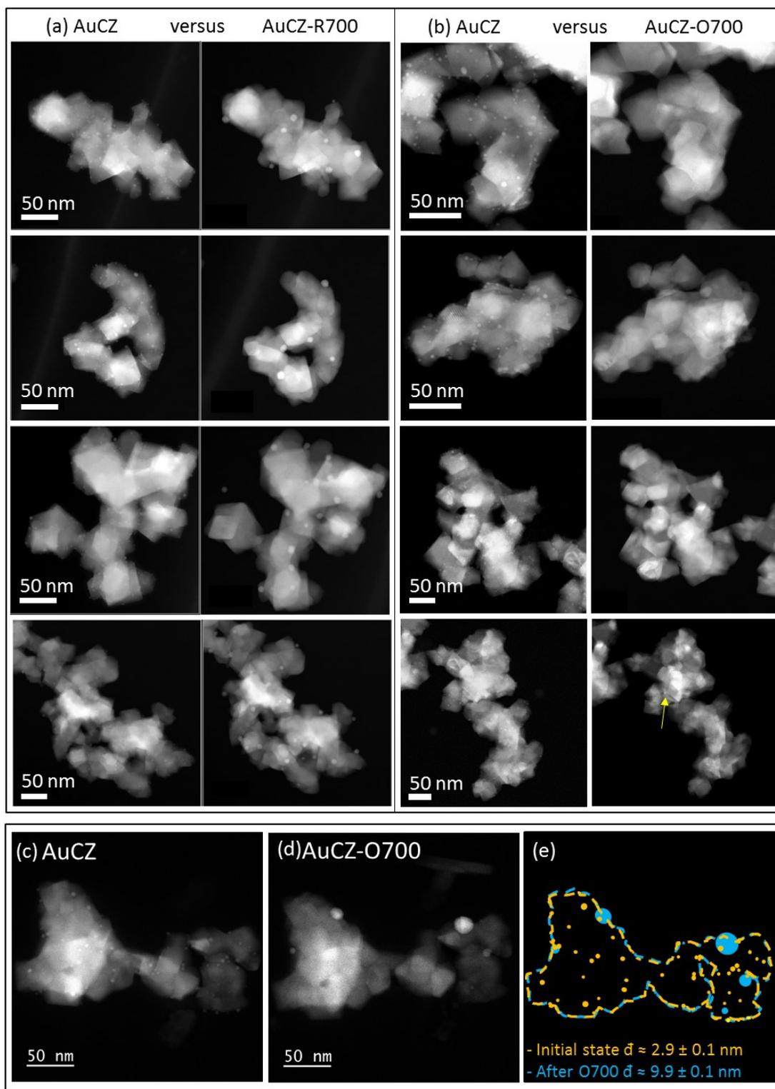
**Figure S1.** Representative Identical Location HAADF-STEM images of gold catalysts at (a) original versus after R700; (b) original versus after O700. In the set of images after O700 only one Au particle marked by arrow was found. (c) Identical Location area after O700 showing sign of Au particle growth
