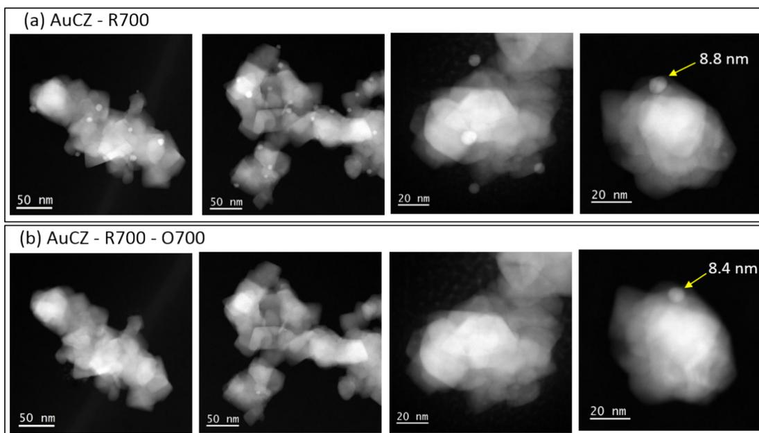
**Figure S7.** Representative Identical Location HAADF-STEM images of gold catalysts at (a) R700 and (b) after O700.
