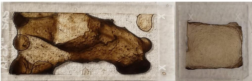
**Supplementary Figure S1.** Example of dopamelanin films prepared by drop-casting. Controlling the film's uniformity is difficult with this method.
