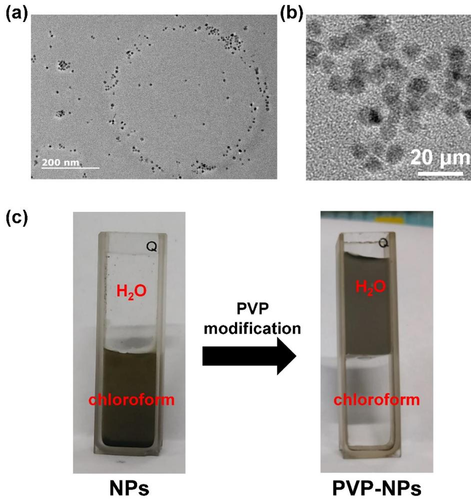
**Fig. S3.** (a, b) TEM of PVP-NPs. (c) Photograph of NPs dispersed in chloroform (left) and in pure water (right) before and after PVP modification.
