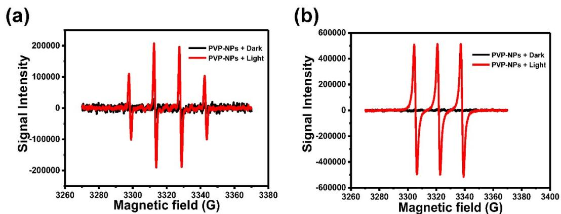
Fig. S7. (a) Electron paramagnetic resonance spectra of PVP-NPs after white light irradiation or not in the presence of DMPO. (b) Electron paramagnetic resonance spectra of PVP-NPs after white light irradiation or not in the presence of TEMP.
