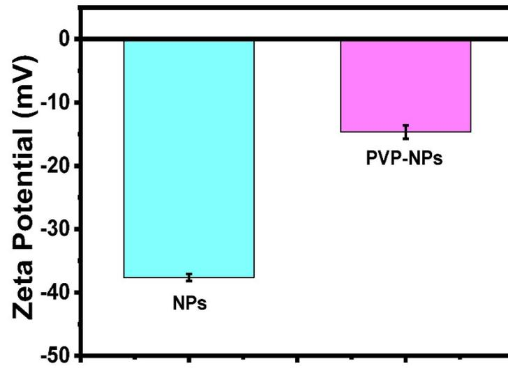
Fig. S4. Zeta potential analysis of NPs and PVP-NPs.
