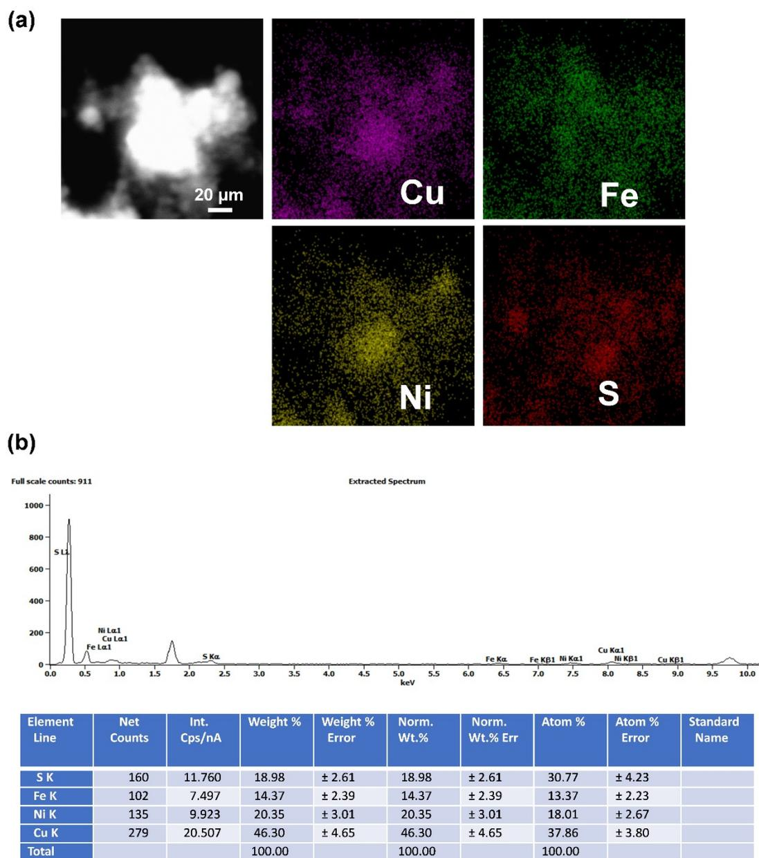
Fig. S1. (a) TEM-EDS mapping and (b) compositional analysis of NPs.
