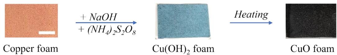
**Fig. S4** Process of the copper foam was oxidized to copper hydroxide and copper oxide and their surface optical images (scale: 1 cm).
