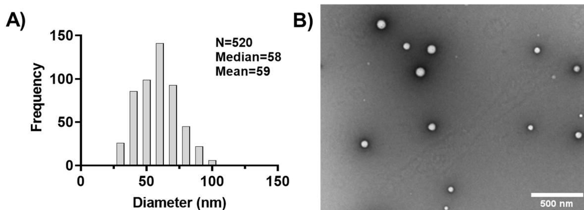
**Figure S3.** TEM characterization of PLGA-PEG NPs.
