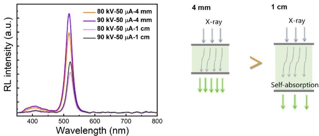
**Figure S18** RL spectra of CsPbBr<sub>3</sub> QDs/PPO LSS with 4 mm and 1 cm thickness (80 kV-50  $\mu$ A and 90 kV-50  $\mu$ A).
