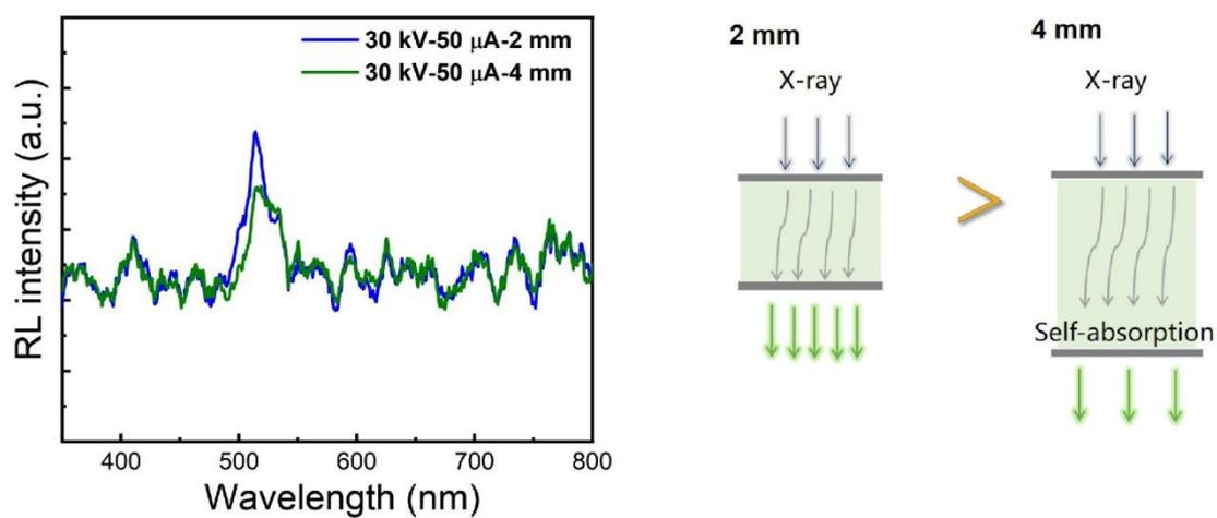
**Figure S16** RL spectra of CsPbBr<sub>3</sub> QDs/PPO LSS with 2 mm and 4 mm thickness (30 kV-50 uA).
