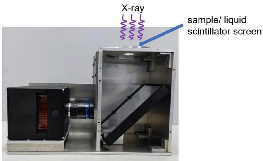
Figure S5 X-ray imaging optical system.
