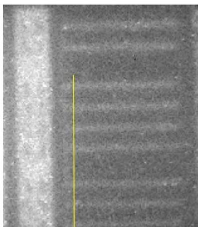
Figure S6. X-ray imaging of the standard line-pair card by the pixelated  $\text{CsPbBr}_3/\text{PPO}$  LSS.
