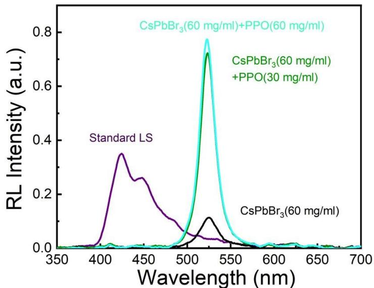
**Figure S15.** RL spectra of standard liquid scintillator (PPO+POPOP+toluene), CsPbBr<sub>3</sub>(60 mg/ml), CsPbBr<sub>3</sub>(60 mg/ml)+PPO (30 mg/ml) and CsPbBr<sub>3</sub>(60 mg/ml)+PPO (60 mg/ml), measured at 90 kV, 89 uA
