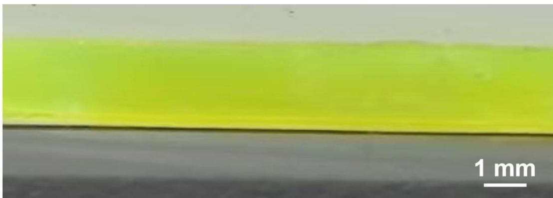
**Figure S1** Cross-sectional image of the pixelated CsPbBr<sub>3</sub>/PPO liquid scintillator arrays
