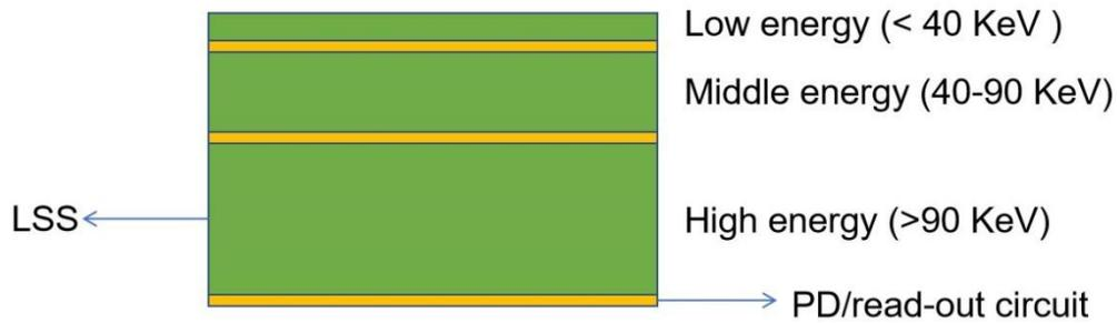
**Figure S19** Schematic diagram of the energy resolved X-ray detector based on the LSS.
