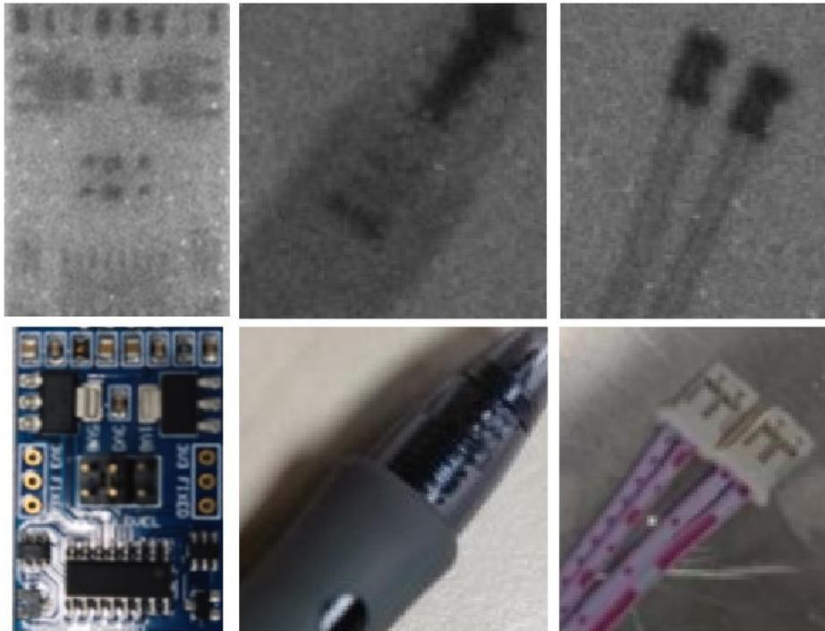
Figure S11. X-ray images and photographs of circuit board, ball-point pen and leadwire using Mn: CsPbCl<sub>3</sub> QDs/PPO LSS.
