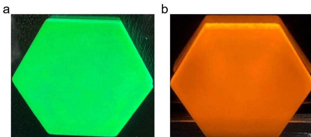
**Figure S14.** (a-b) Optical image of the pixelated CsPbBr<sub>3</sub>/PPO and Mn:CsPbCl<sub>3</sub> QDs/PPO liquid scintillator arrays under UV light excitation after the repeated filling/packaging process, respectively.
