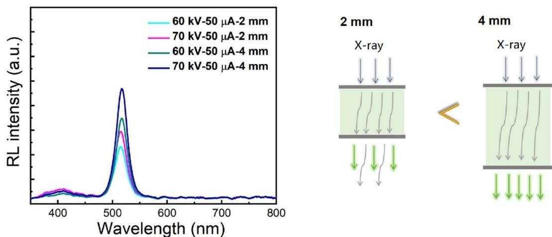
**Figure S17** RL spectra of CsPbBr<sub>3</sub> QDs/PPO LSS with 2 mm and 4 mm thickness (60 kV-50  $\mu$ A and 70 kV-50  $\mu$ A).
