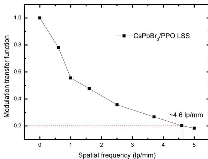
Figure S7. Modulation transfer function (MTF) of CsPbBr<sub>3</sub> QDs/PPO LSS
