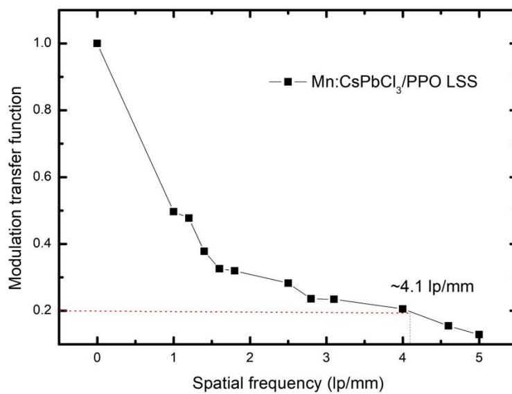
**Figure S13.** MTF of Mn:CsPbCl<sub>3</sub> QDs/PPO LSS
