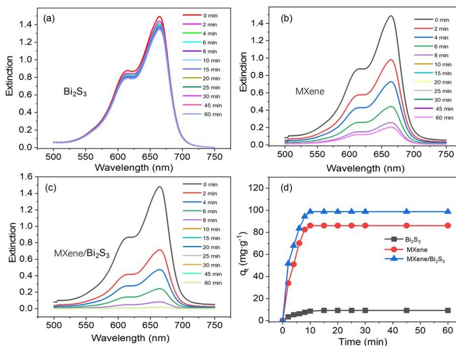
**Figure S10.** Time-dependent extinction spectra of MB in the presences of  $\text{Bi}_2\text{S}_3$  (a), MXene (b), and MXene/ $\text{Bi}_2\text{S}_3$  (c). (d) The comparison of adsorption abilities of  $\text{Bi}_2\text{S}_3$ , MXene, and MXene/ $\text{Bi}_2\text{S}_3$ .
