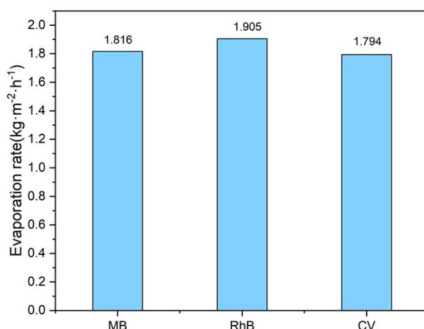
**Figure S8.** Evaporation rates of MXene/Bi<sub>2</sub>S<sub>3</sub> membrane measured in MB, RhB, and CV solution.
