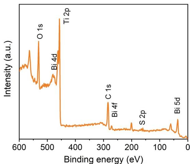
**Figure S1.** XPS survey of MXene/ $\text{Bi}_2\text{S}_3$  hybrids.
