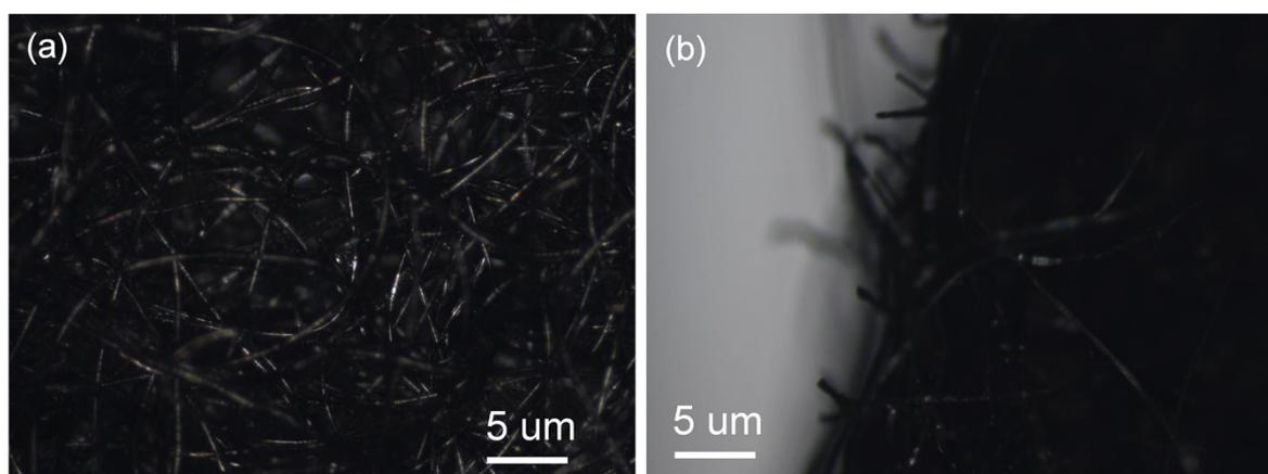
**Figure S3.** Optical images of MXene/ $\text{Bi}_2\text{S}_3$  hybrids observed on top view (a) and side view (b).
