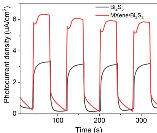
**Figure S2.** Photocurrent densities of  $\text{Bi}_2\text{S}_3$  and MXene/ $\text{Bi}_2\text{S}_3$  electrodes under light irradiation. In the measurements, Pt electrode and AgCl electrode were used as counter electrode and reference electrode,  $\text{Na}_2\text{SO}_4$  (1 M) was used as electrolyte.
