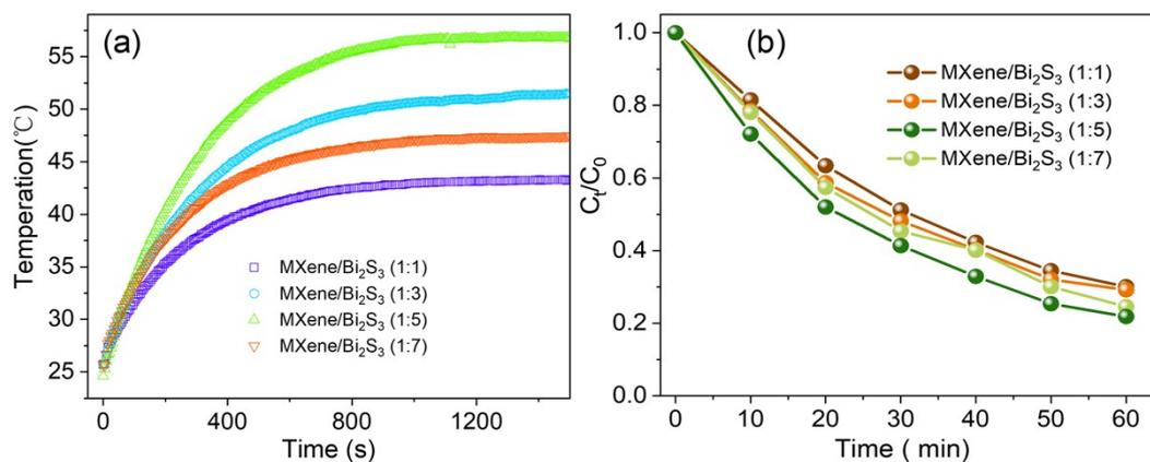
**Figure S9.** Temperature variation curves (a) under an 808 nm laser irradiation and
