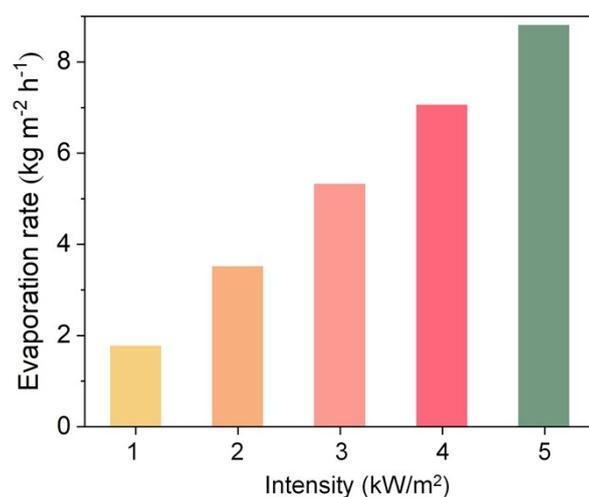
**Figure S7.** Mass change of water in the presence of MXene/Bi<sub>2</sub>S<sub>3</sub> membrane under sunlight irradiation with different intensities.
