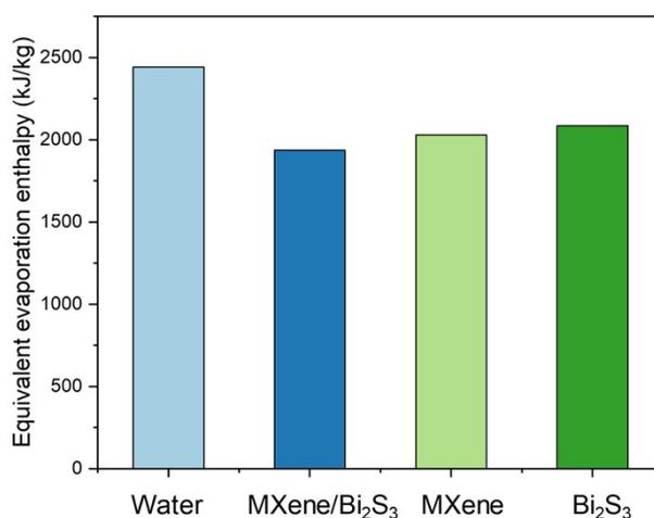
**Figure S6.** Equivalent vaporization enthalpy of Bi<sub>2</sub>S<sub>3</sub>, MXene, and MXene/Bi<sub>2</sub>S<sub>3</sub> membranes. The calculation is based on the formula  $\Delta H_0 m_0 = \Delta H_{equ} m_g$ , where  $\Delta H_0$  is the evaporation enthalpy of pure water,  $m_0$  is the spontaneous evaporation rate of water in dark,  $m_g$  is spontaneous evaporation rate of membrane,  $\Delta H_{equ}$  is the equivalent vaporization enthalpy.
