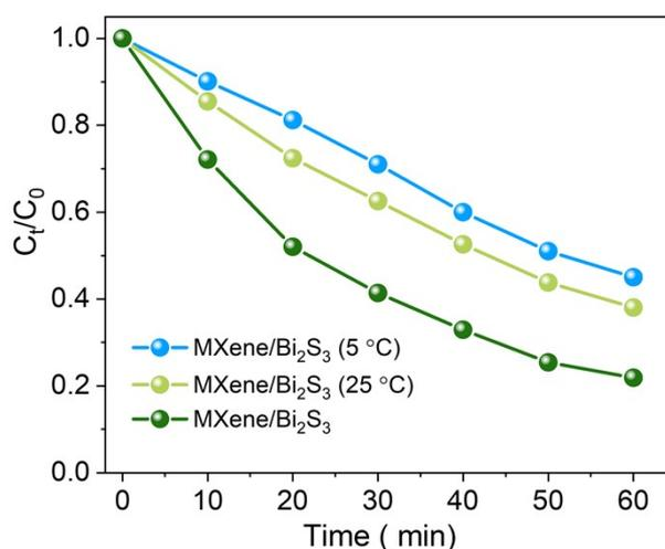
**Figure S11.** The photocatalytic degradation of MB of MXene/ $\text{Bi}_2\text{S}_3$  measured at different temperature controlled by cooling water.
