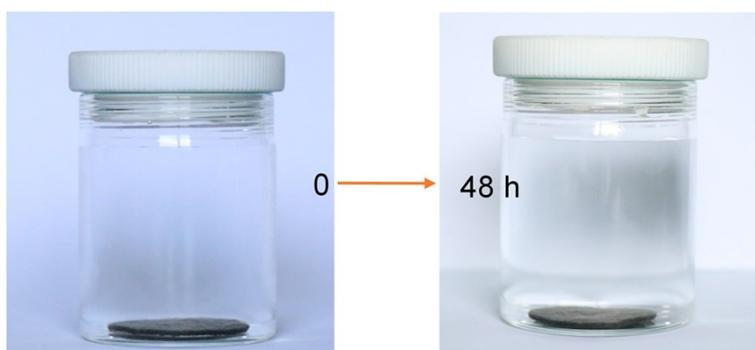
**Figure S4.** Photographs of MXene/Bi<sub>2</sub>S<sub>3</sub> membrane soaking in water for 48 h.
