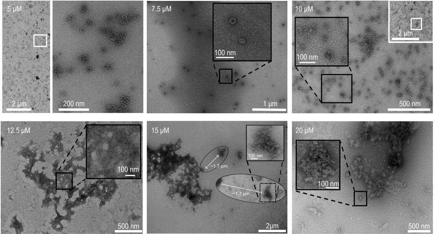
Fig. S1 TEM images of the same samples as shown in Fig. 4, but at different magnifications for each sample (some rotation and translation may be present between the low-magnification images and the insets due to drift in the microscope). The low magnification images of the samples at 12.5  $\mu\text{M}$  coat-protein dimer concentration and higher show micrometer-sized structures.
