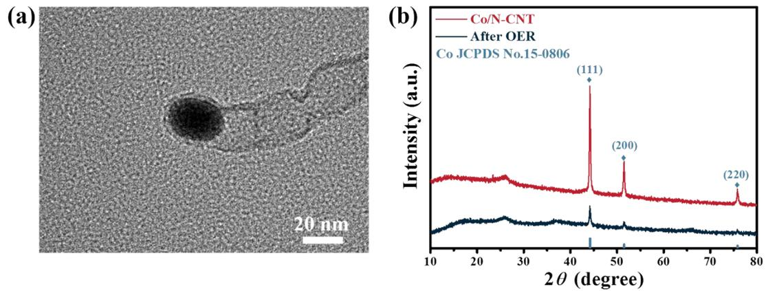
**Fig. S9** (a) TEM images of Co/N-CNT after OER stability tests, (b) XRD patterns of Co/N-CNT before and after OER stability testing.
