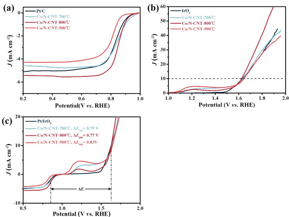
**Fig. S5** LSV curves of 20% Pt/C, Co/N-CNT-700 °C, Co/N-CNT-800 °C, and Co/N-CNT-900 °C during (a) ORR and (b) OER; (c) The ORR/OER bifunctional LSV curves.
