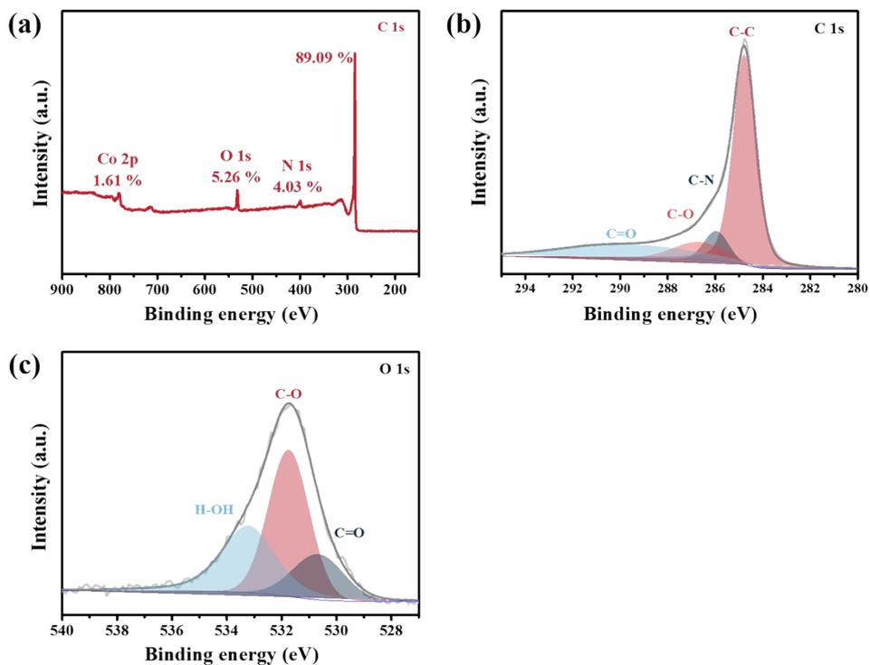
Fig. S4 (a) Full survey XPS spectrum and high-resolution XPS spectra of (b) C 1s and (c) O 1s of the Co/N-CNT.
