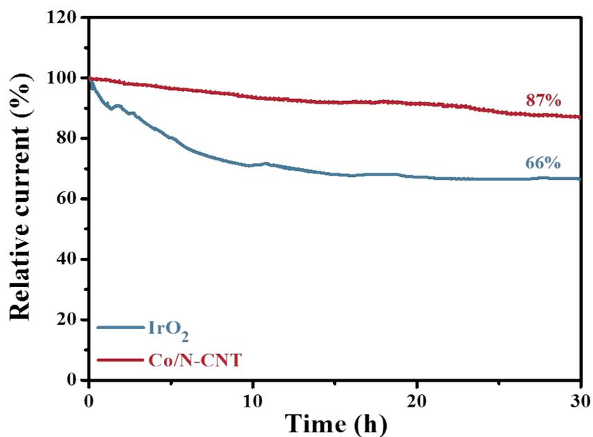
**Fig. S8** Chronoamperometry curves of Co/N-CNT and IrO<sub>2</sub> electrocatalysts in O<sub>2</sub>-saturated 0.1 M KOH electrolyte.
