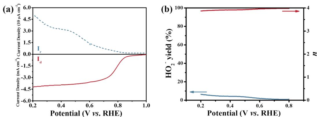
**Fig. S6** (a) RRDE voltammograms of Co/N-CNT at 1600 rpm in 0.1 M KOH. (b) HO<sub>2</sub><sup>-</sup> yield (%) and electron transfer number ( $n$ ) according to the RRDE measurements in 0.1 M KOH.
