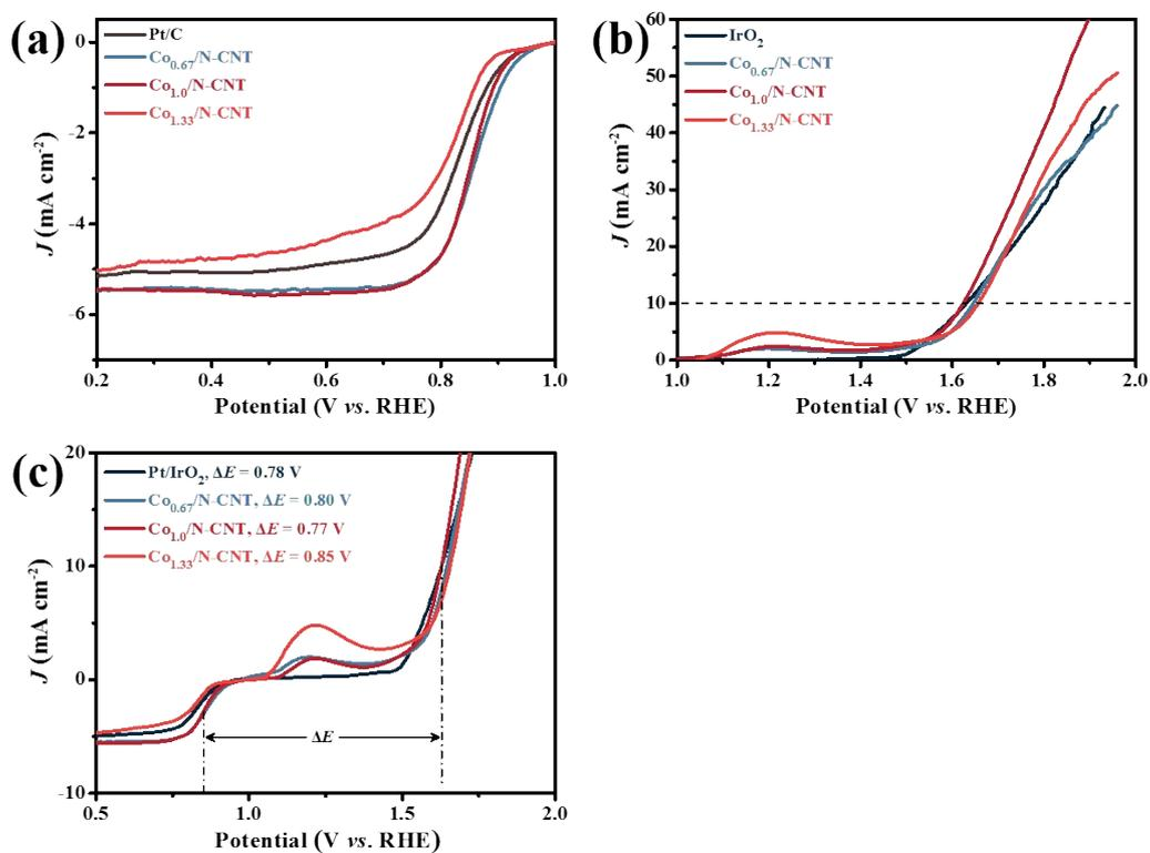
**Fig. S2** LSV curves of 20% Pt/C, Co<sub>0.67</sub>/N-CNT, Co<sub>1.0</sub>/N-CNT, and Co<sub>1.33</sub>/N-CNT electrocatalysts during ORR (a) and (b) OER; (c) The ORR/OER bifunctional LSV
