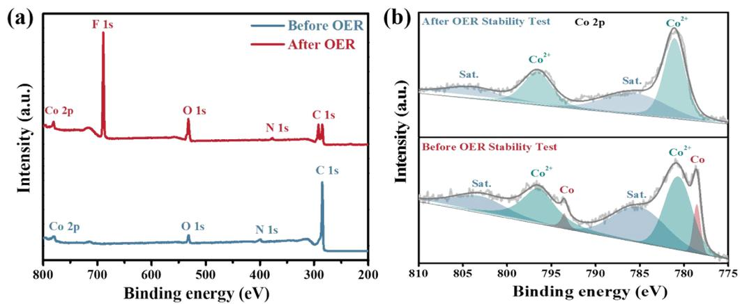
**Fig. S10** (a) Full survey XPS spectrum and (b) high-resolution XPS spectra of Co 2p, of Co/N-CNT before and after OER stability test.
