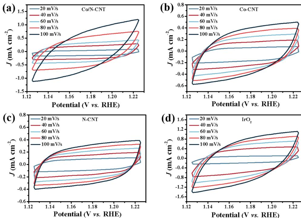
**Fig. S7** Cyclic voltammetry (CV) curves of (a) Co/N-CNT, (b) Co-CNT, (c) N-CNT, and (d) IrO<sub>2</sub> in O<sub>2</sub>-saturated 1.0 M KOH solution at different scan rates.
