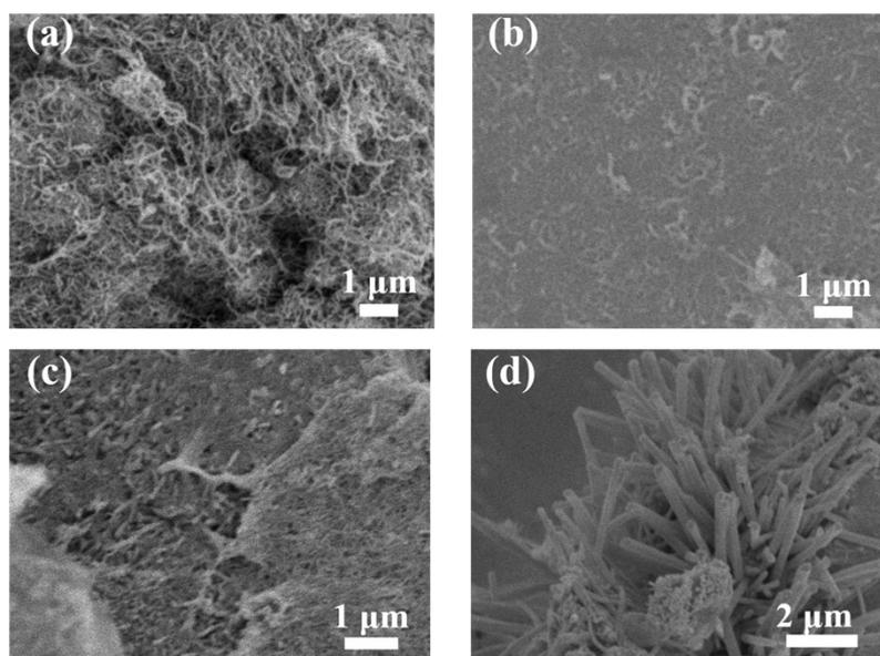
**Fig. S1** SEM images of (a) MWCNT, (b) HMWCNT, (c) Co<sub>0.67</sub>-Mel-HMWCNT and (d) Co<sub>1.33</sub>-Mel-HMWCNT.
