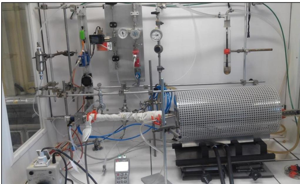
Figure S1. Chemical Vapor Deposition set-up
