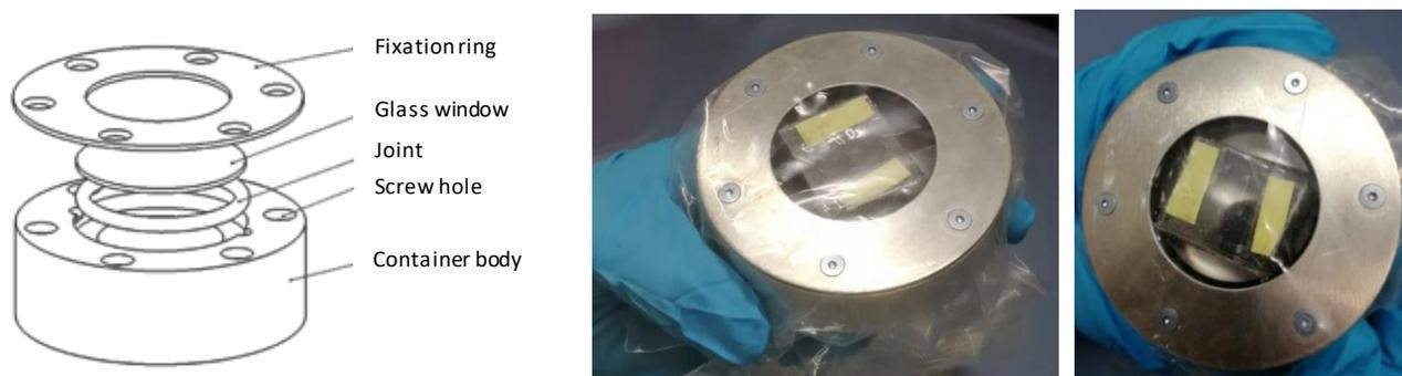
Figure S18. Container designed to confine <sup>14</sup>C-Graphite while running the Raman experiment
