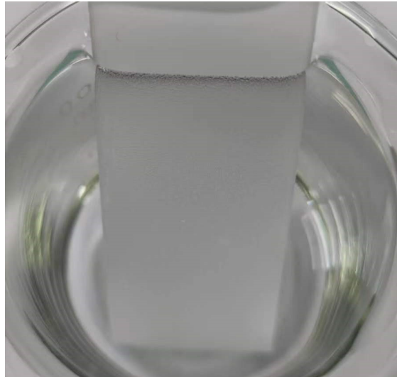
Figure S8. Optical image: Air pocket formed by micron and nanometre rough structure in liquid.
