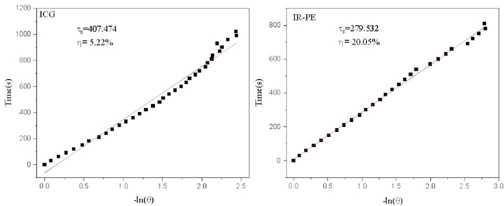
**Figure S8.** Photothermic heating curves of ICG and IR-PE solutions under 808 nm irradiation ( $0.1 \text{ W/cm}^2$ ) for 10 min followed by cooling to room temperature. Linear correlation of the cooling times versus negative natural logarithm of driving force temperatures.
