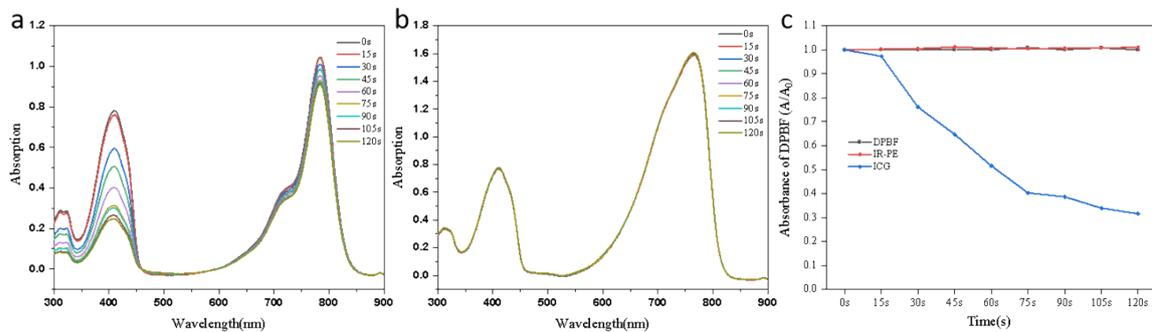
**Figure S9.** Absorption spectra of ICG ( $10 \text{ µg/mL}$ ) (a) and IR-PE ( $10 \text{ µg/mL}$ ) (b) in PBS (pH 3.5) containing DPBF ( $50 \text{ µM}$ ) upon 808 nm irradiation ( $0.1 \text{ W/cm}^2$ ). (c) Comparison of ROS generation of ICG and IR-PE in PBS under upon 808 nm irradiation ( $0.1 \text{ W/cm}^2$ ) for 120 s.
