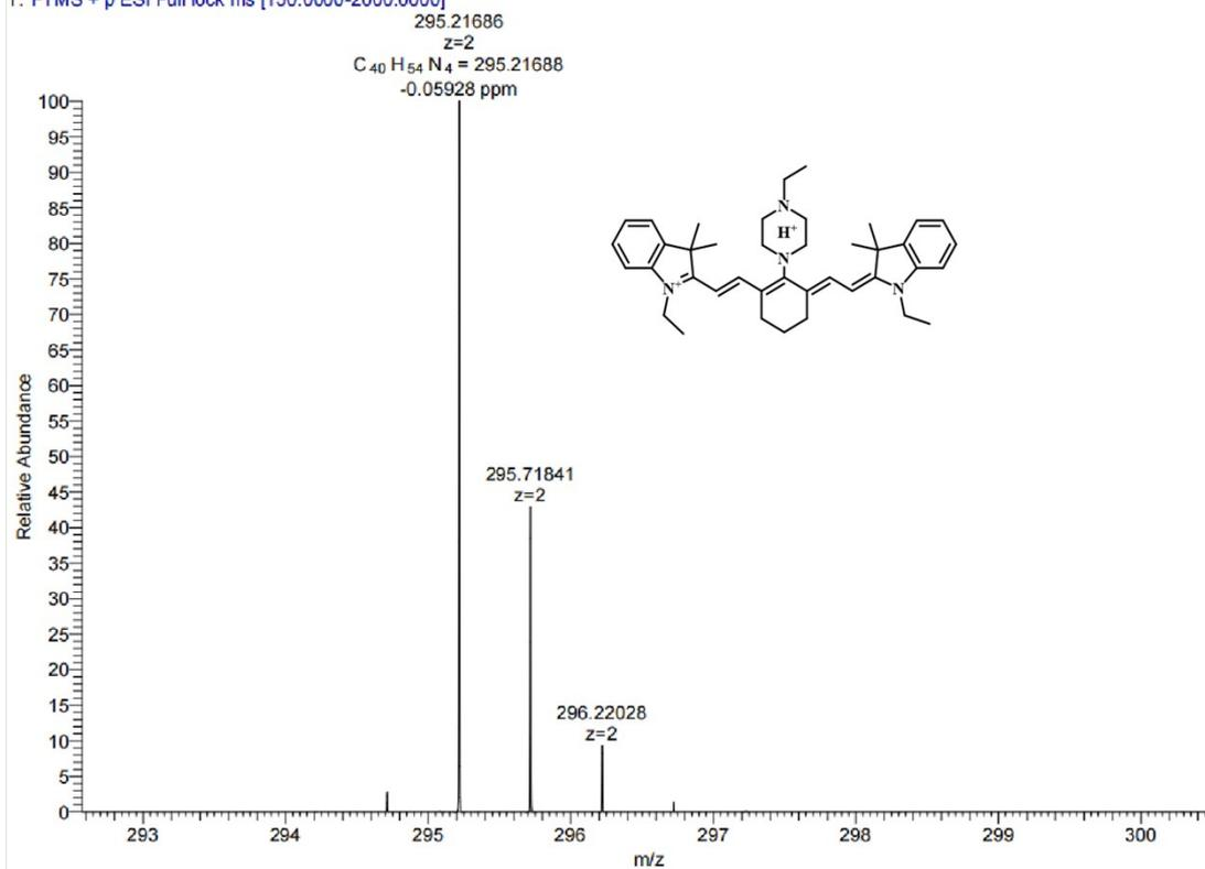
**Figure S5.** High resolution mass spectrum (MALDI-TOF) of IR-PEH.
