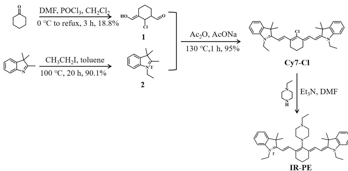
**Figure S1.** Synthetic route to IR-PE.
