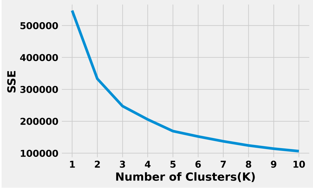
Figure S3: SSE-vs-Number of Clusters(K). The point of inflection lies at K=3
