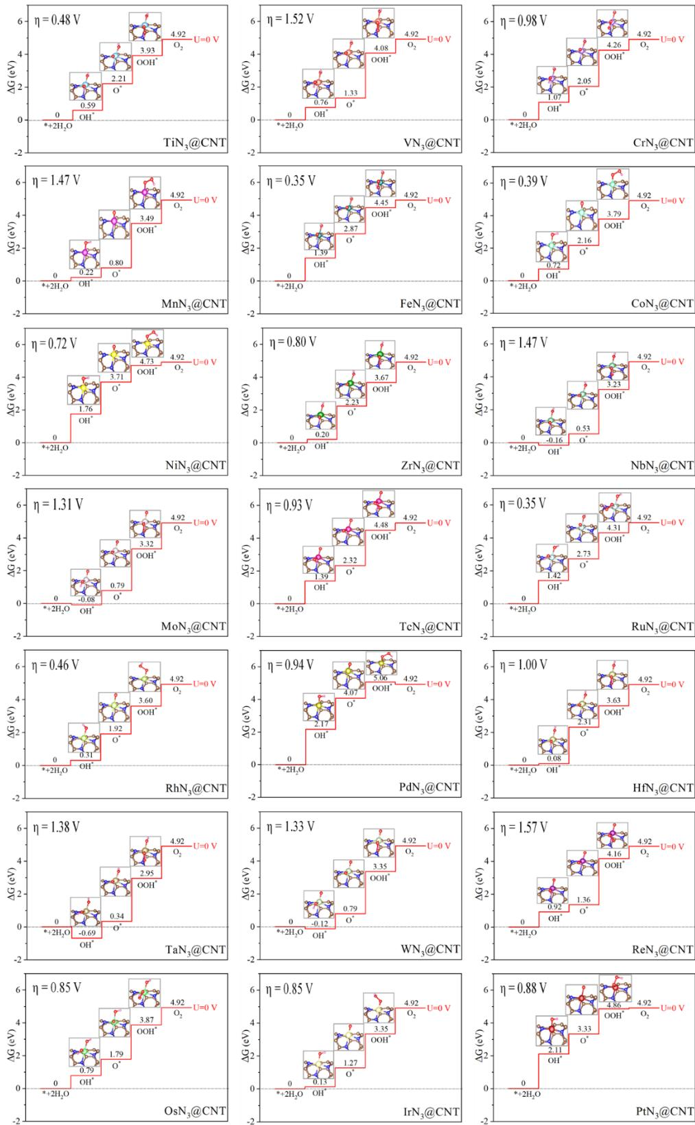
**Fig. S7** Gibbs free energy diagram of OER for TMN<sub>3</sub>@CNT series.
