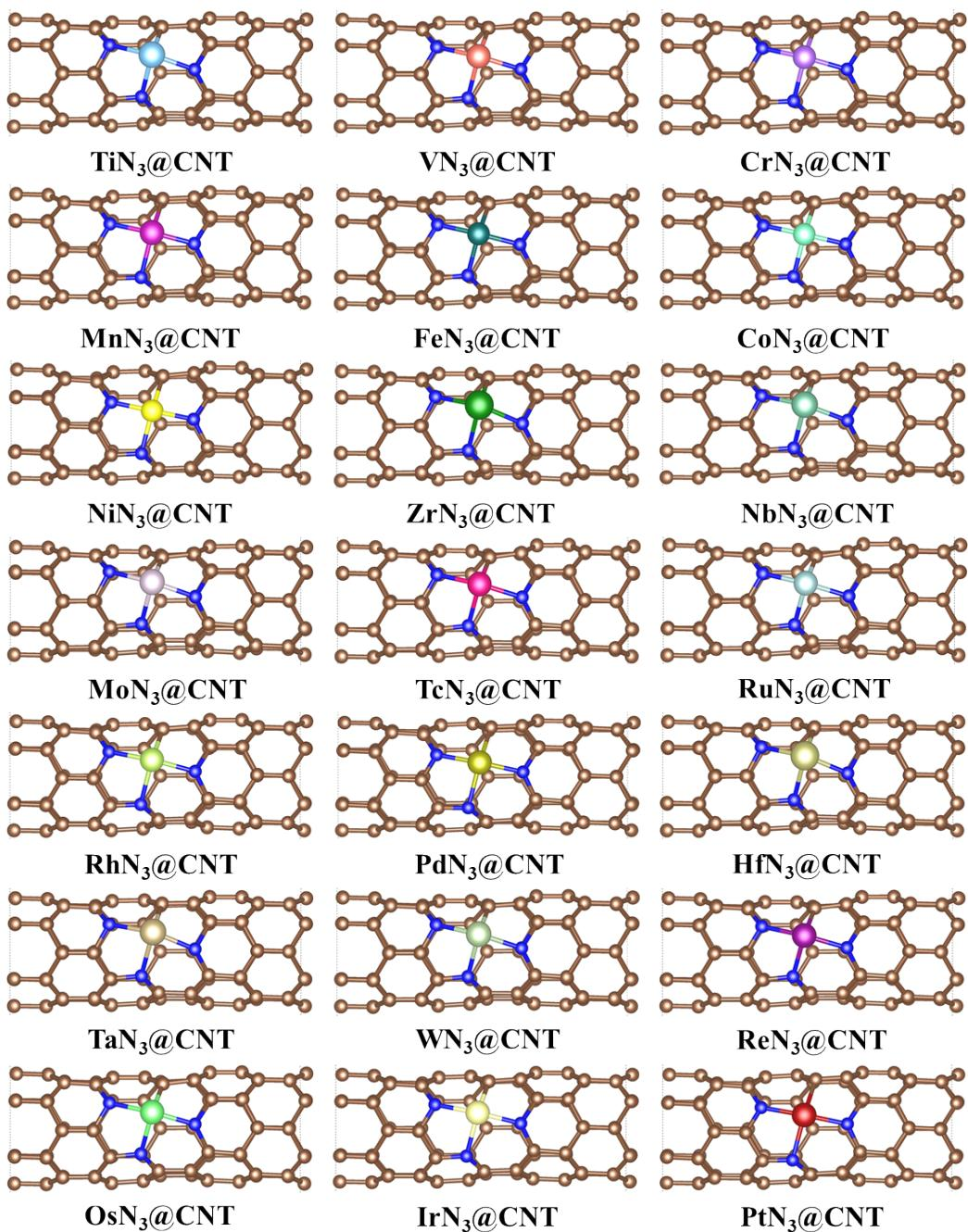
**Fig. S3** The optimized structures of  $\text{TMN}_3@\text{CNT}$  ( $\text{TM} = \text{Ti}, \text{V}, \text{Cr}, \text{Mn}, \text{Fe}, \text{Co}, \text{Ni}, \text{Zr}, \text{Nb}, \text{Mo}, \text{Tc}, \text{Ru}, \text{Rh}, \text{Pd}, \text{Hf}, \text{Ta}, \text{W}, \text{Re}, \text{Os}, \text{Ir}$  and  $\text{Pt}$ ).
