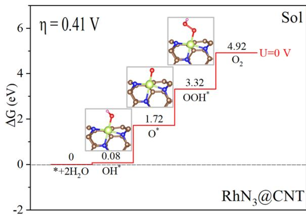
**Fig. S1** The free energy diagram of OER in solvation for the sampled RhN<sub>3</sub>@CNT.
