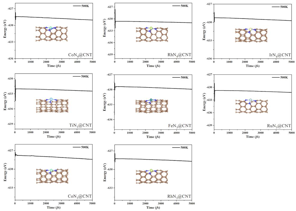
**Fig. S8** Ab initio molecular dynamics simulation for the  $\text{TMN}_x\text{@CNT}$  ( $x = 3$  and 4) systems with high OER catalytic activity and their corresponding morphologies after  $5000\text{ fs}$  at  $T=500\text{ K}$ .
