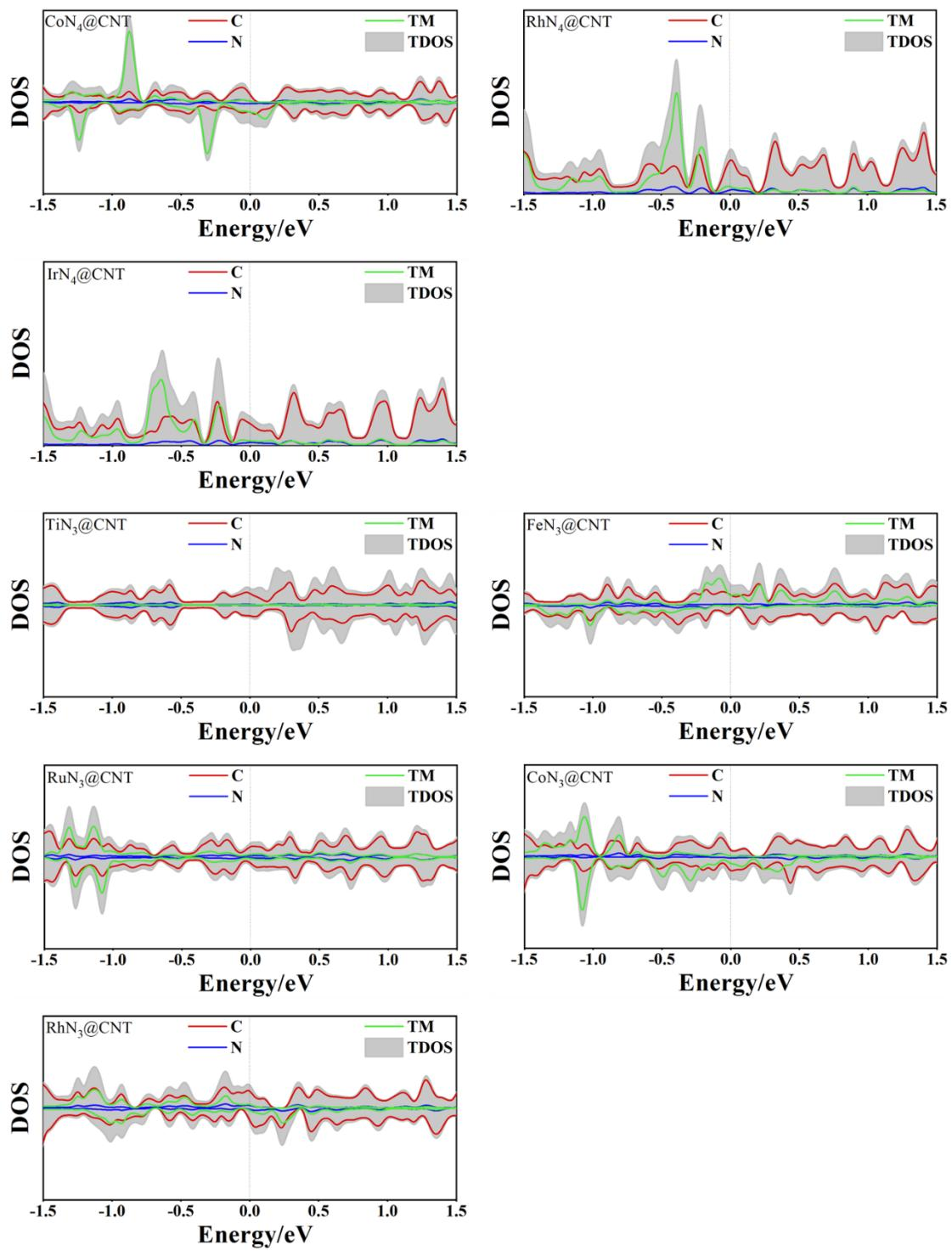
**Fig. S9** Density of states for  $\text{TMN}_x@\text{CNT}$  ( $x = 3$  and  $4$ ) systems with high OER catalytic activity.
