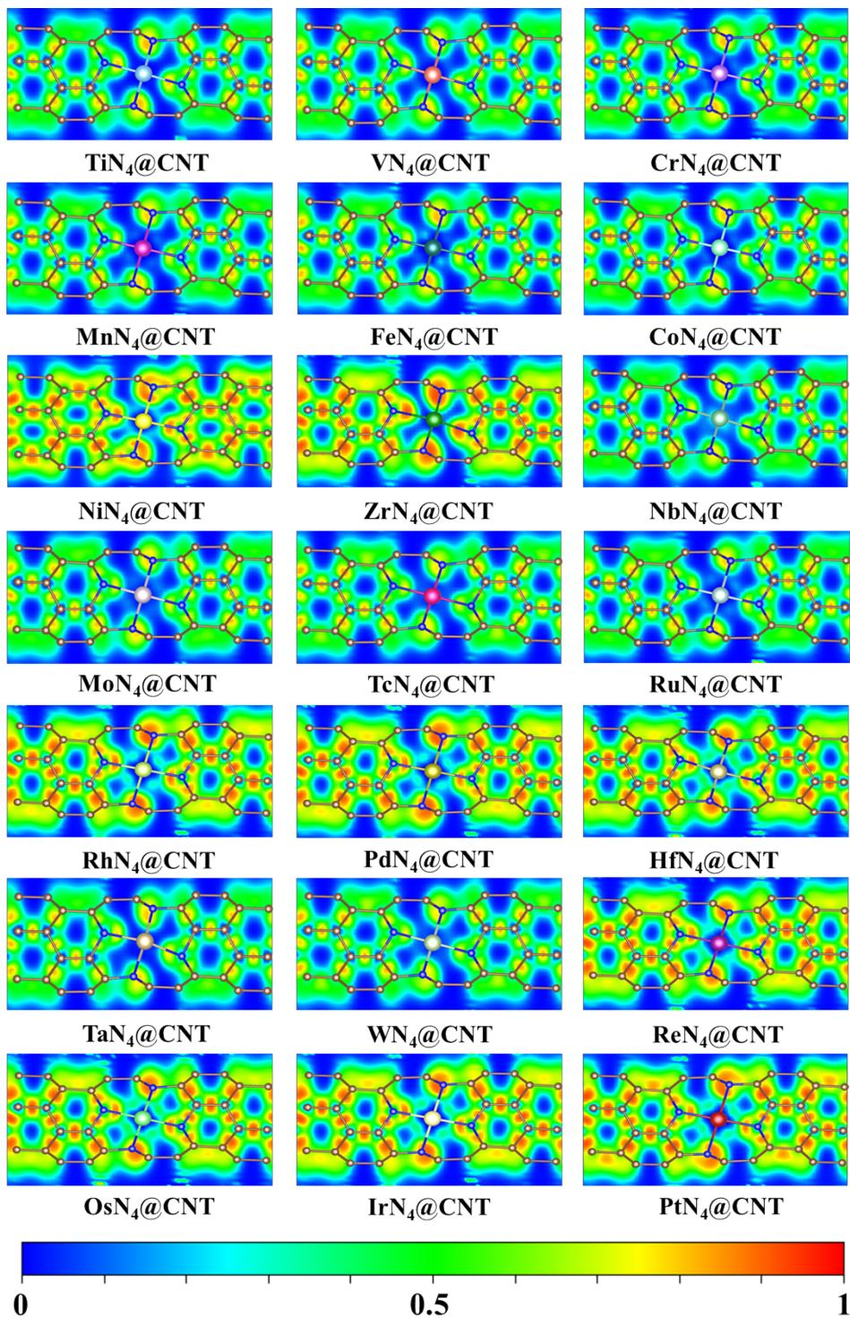
**Fig. S4** Plots of electron location function (ELF) for TMN<sub>4</sub>@CNT systems. Note that ELF can be characterized in the form of a contour plot within a range of 0-1. The region close to 1 indicates the presence of covalent electrons or lone-pair electrons; the region of 0.5 represents homogenous electron gas; and the region near to 0 suggests a low electron density area.
