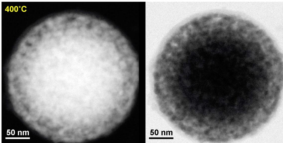
Movie S3. HAADF-STEM (left) and ABF-STEM (right) images of the NiO/YSZ/BZY nanocomposite particle being heated from 400°C to 900°C in H<sub>2</sub> gas showing the continuous morphological changes.
