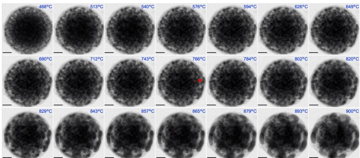
Figure S2. A series of ABF-STEM images of an isolated NiO/YSZ/BZY nanocomposite particle being heated from 400°C to 900°C in H<sub>2</sub> gas (the gas pressure is 1 atm). Gradually coarsening of primary particles on the outer surface of the composite particle can be obviously identified from 766°C. The scale bar is 50 nm.
