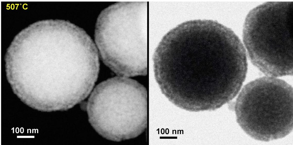
Movie S6. HAADF-STEM (left) and ABF-STEM (right) images of the NiO/YSZ/BZY nanocomposite particles being heated from 400°C to 900°C in H<sub>2</sub> gas showing the migrating of Ni atoms along the external surfaces, and eventually congregating at the grain boundary triple point where the NiO/YSZ/BZY nanocomposite particles had formed.
