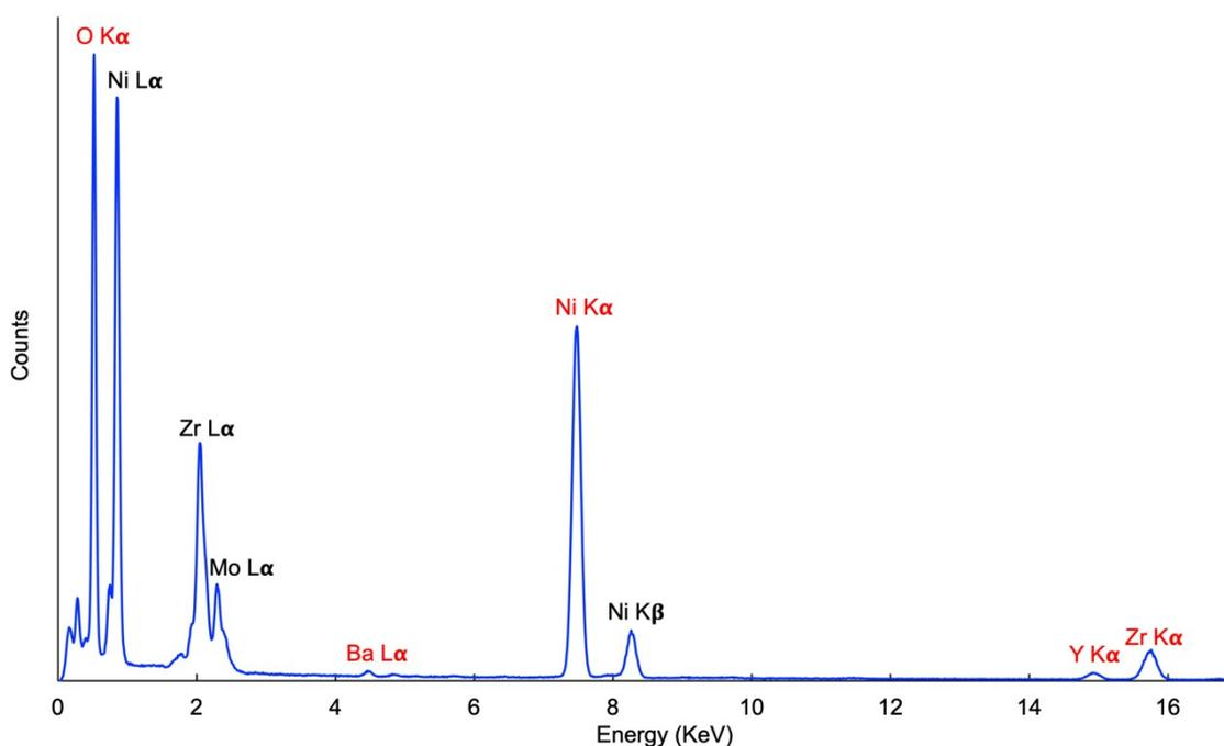
Figure S1. Energy-dispersive X-ray spectroscopy (EDS) spectrum obtained from the designated rectangular region, as indicated in Figure 2h. The red labels highlight the Zr K $\alpha$ , Ni K $\alpha$ , Y K $\alpha$ , O K $\alpha$ , and Ba L $\alpha$  peaks, which were used to generate the elemental maps presented in Figure 2c-2g. The presence of Mo L $\alpha$  peak is attributed to the Mo TEM gird.
