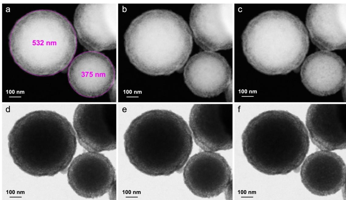
Figure S4. HAADF-STEM (a-c) and the corresponding ABF-STEM images (d-f) of NiO/YSZ/BZY nanocomposite particles heated in N<sub>2</sub> gas environment with a gas pressure of 1 atm. (a) and (d) 300°C; (b) and (e) 700°C; (c) and (f) 900°C.
