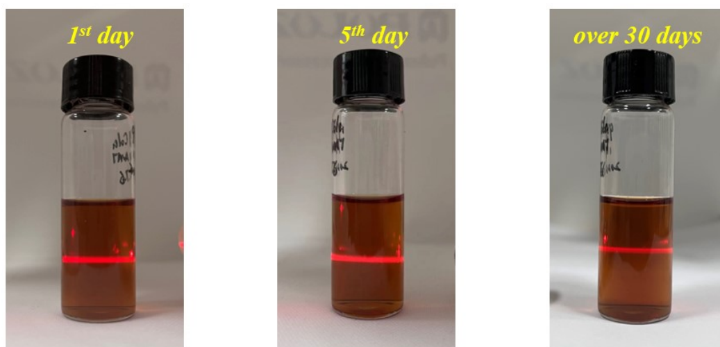
Fig. S1 The digital photographs of the colloidal precursor after being left for different periods of time.
