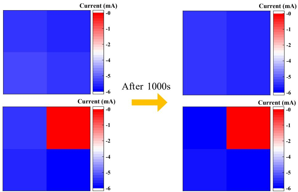
**Fig. S8** The currents within a  $2 \times 2$  cross array were observed over a 1000 s duration, showcasing the endurance of the maintained resistance state in OHP RRAMs.
