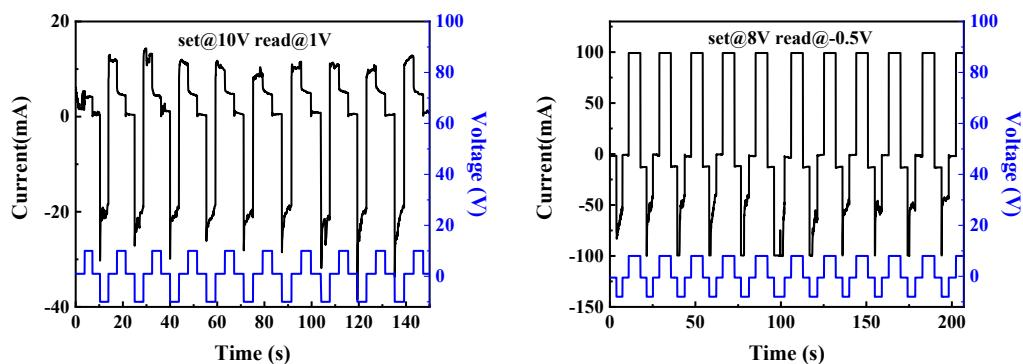
**Fig. S9** Multiple writing-erasing processes of the nonvolatile OHP RRAMs.
