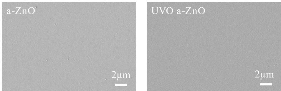
**Fig. S1** Top-view SEM images of UV-treated and untreated a-ZnO films
