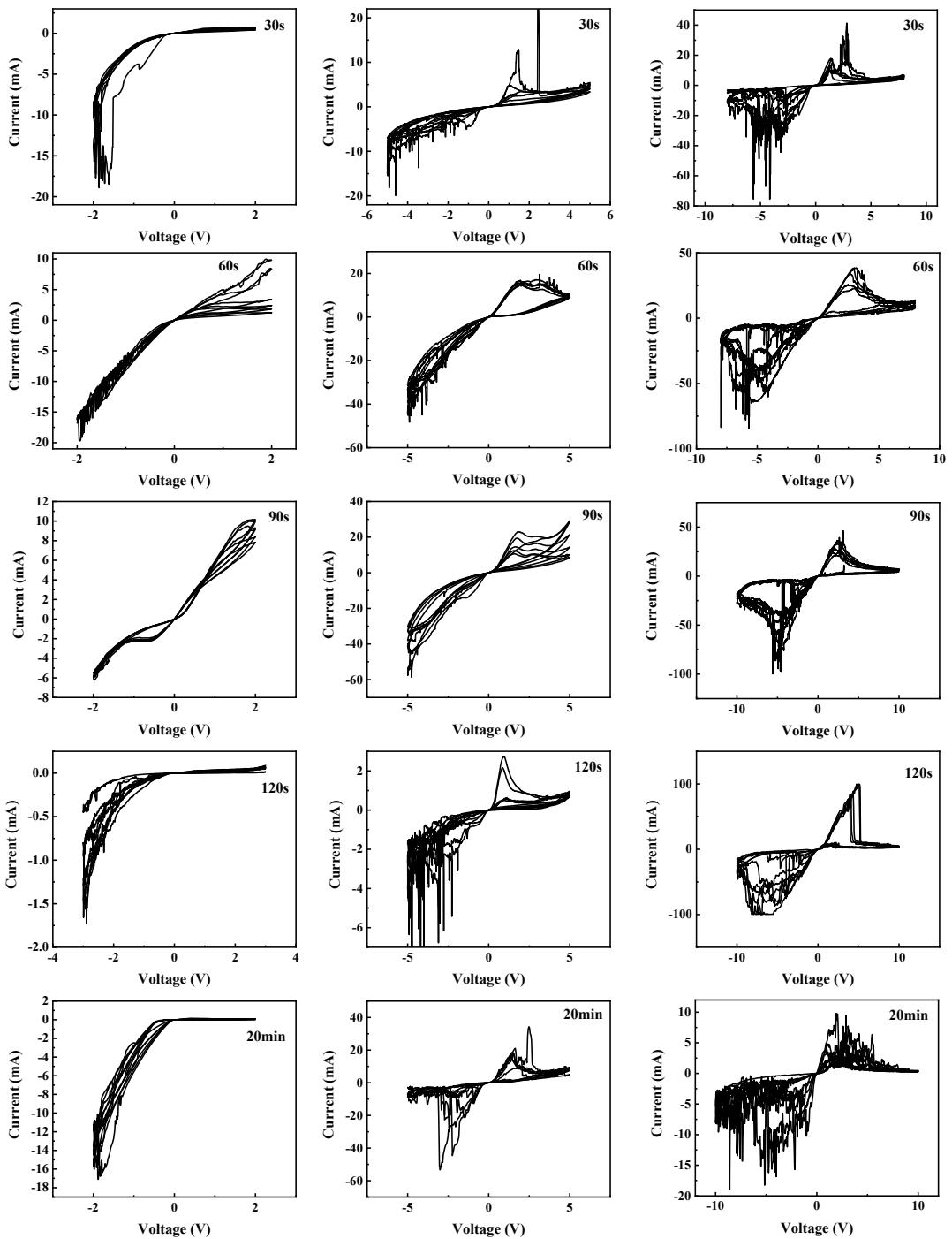
**Fig. S7** A series of RS behaviors of UVO-treated devices under various voltage amplitudes and different treatment times.
