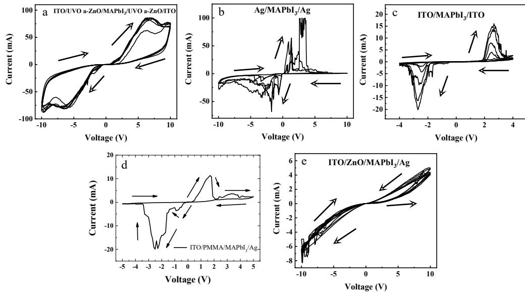
**Fig. S6** Resistive switching behaviors of ITO/ a-ZnO/ MAPbI<sub>3</sub>/ a-ZnO/ ITO, Ag/MAPbI<sub>3</sub>/Ag, ITO/ MAPbI<sub>3</sub>/ ITO, ITO/ PMMA/ MAPbI<sub>3</sub>/ Ag, and ITO/ ZnO (crystal)/ MAPbI<sub>3</sub>/ ITO.
