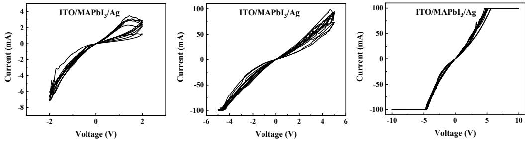
**Fig. S5** I-V characteristics of ITO/ MAPbI<sub>3</sub>/Ag tested by different amplitude of voltages.
