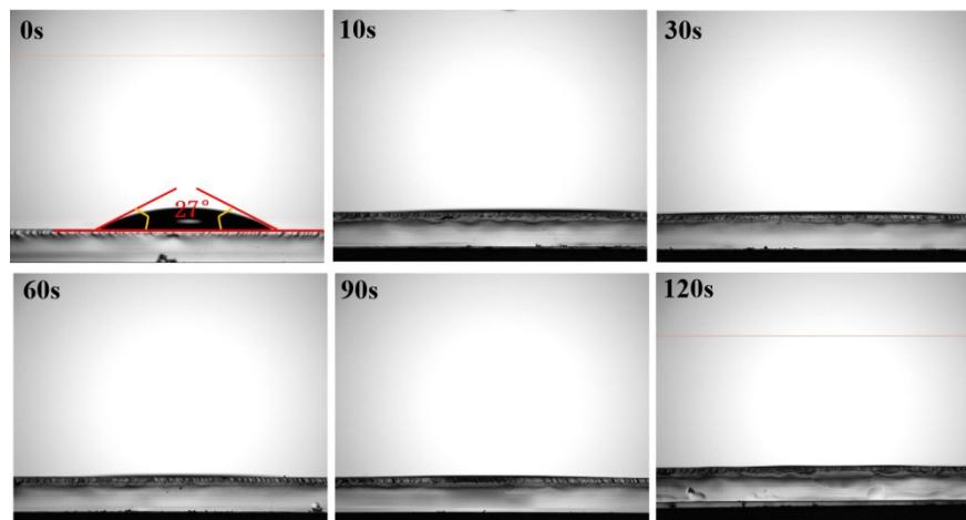
**Fig. S2** DMSO: DMF solution contact angle on a-ZnO films with verious UV-treated time
