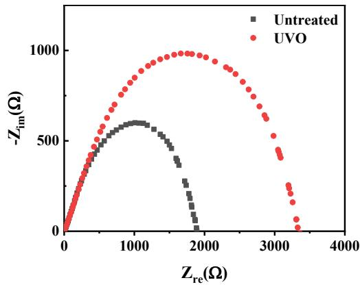
**Fig. S3** The IS spectra evolution of the untreated device and the UVO-treated device.
