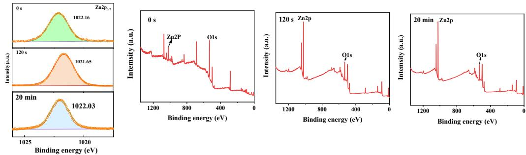
**Fig. S4** High-resolution Zn 2p<sub>3/2</sub> XPS core level spectrum and the full spectrum
