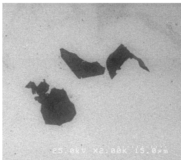
Figure SI 2. A typical scanning electron microscopy (SEM) image of \text{H}_3\text{Sb}_3\text{P}_2\text{O}_{14} nanosheets.
